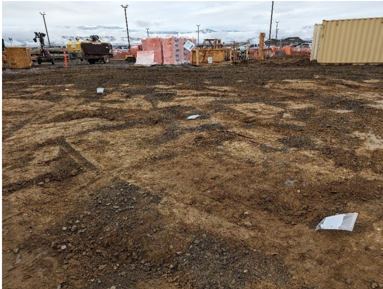
Field screening samples were collected in resealable plastic bags and evaluated for petroleum impact.
