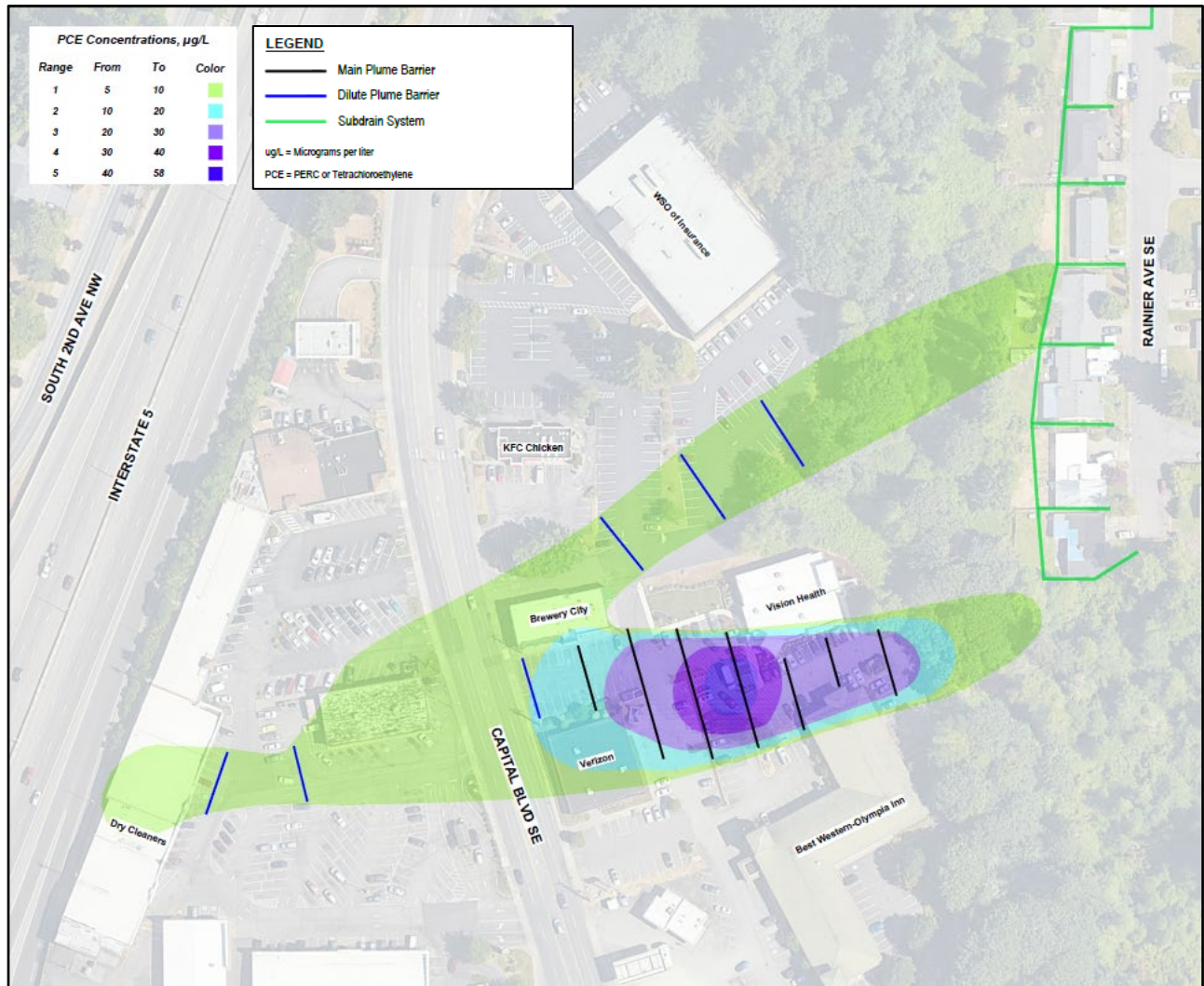
Figure 11. Conceptual Barrier Layout for Alternatives 5: SVE and In Situ Sequestration and Alternative 6: SVE and In Situ Sequestration with ISCR
