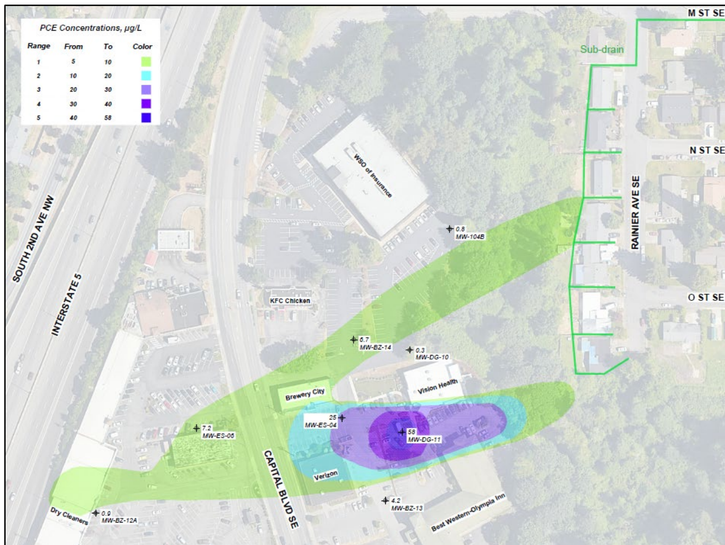
Figure 5. PCE Groundwater Plume and Sub-Drain – Spring 2021
