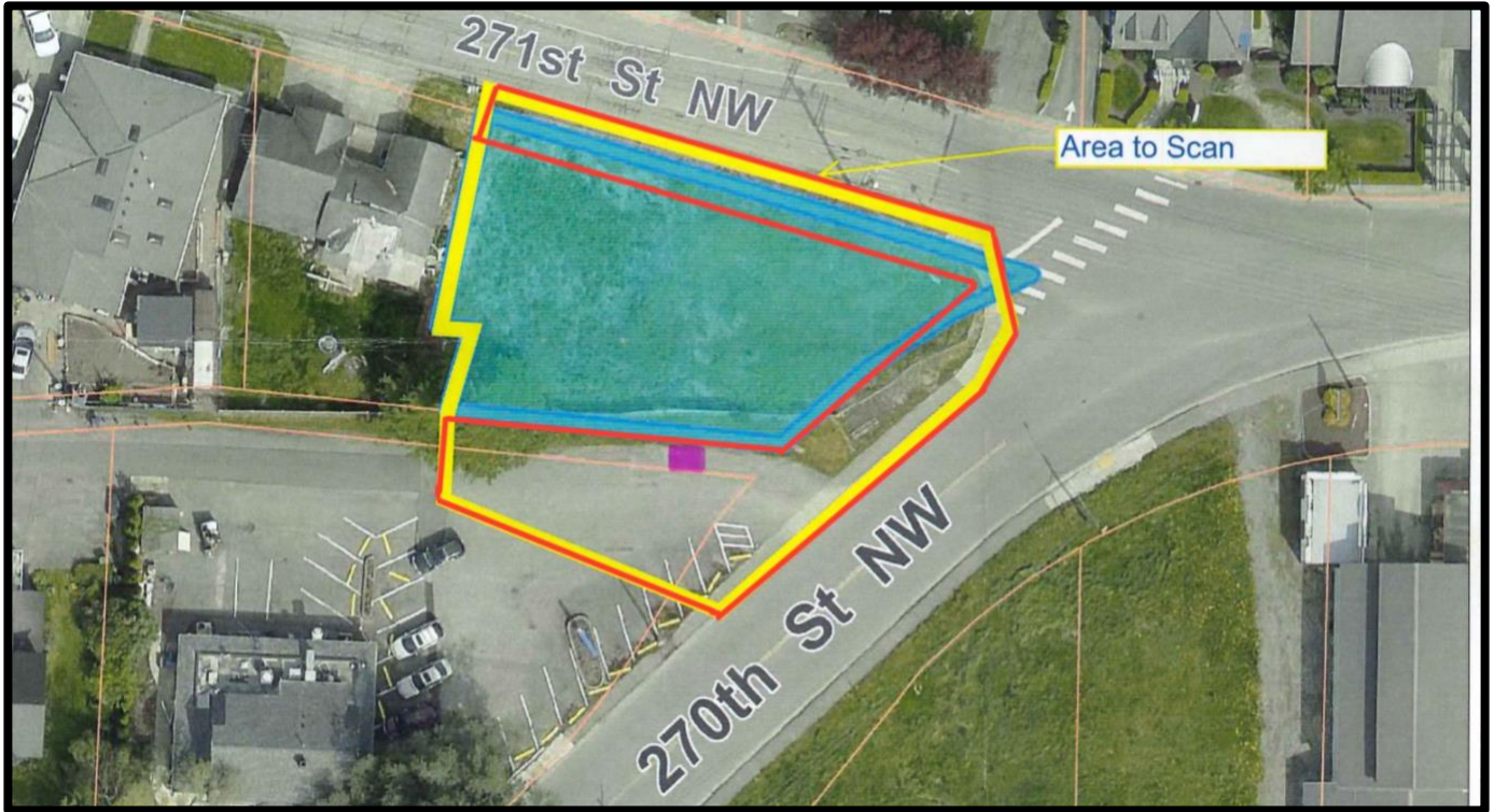
Image 1: Site map with the extent of the requested area bordered in yellow, and the approximate extent of the area scanned on this date bordered in red. The blue border indicates the approximate boundary of the fence line. The pink highlighted area indicates the approximate location of observed UST indications.
