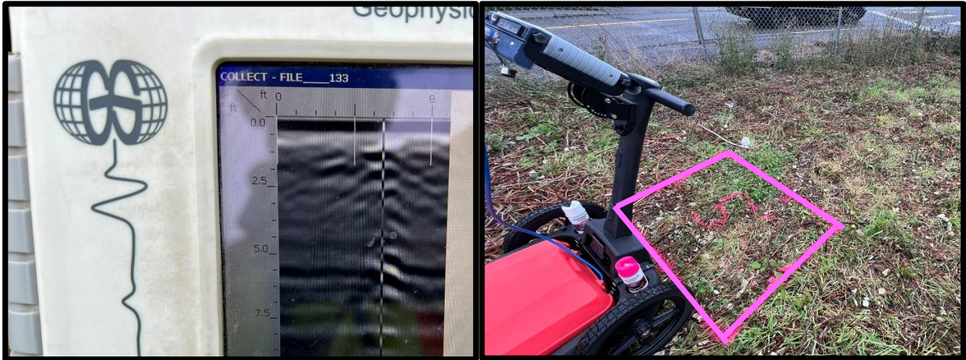
Image 6: GPR cross-section with vertical reference line centered on Anomaly 5 (left). Its observed extent is outlined in pink (right).
