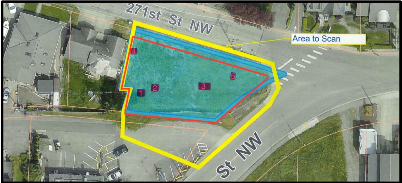
Image 1: Site map with the extent of the requested area bordered in yellow, and the approximate extent of the area scanned on this date bordered in red. The blue border indicates the approximate boundary of the fence line. The approximate location of subsurface anomalies identified on this date are marked and numbered in pink .
