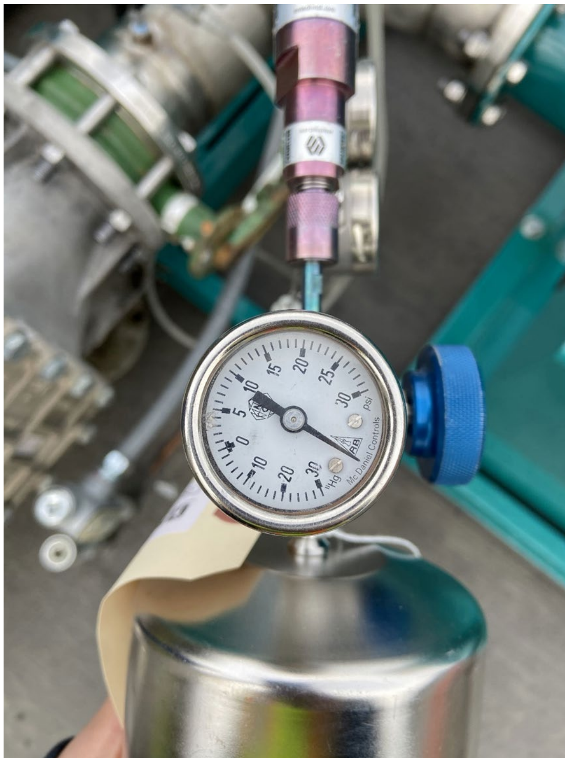
Figure 4. Pressure Gauge for North Blower Sampling with Initial Vacuum of Greater than 30 Inches of Mercury.
