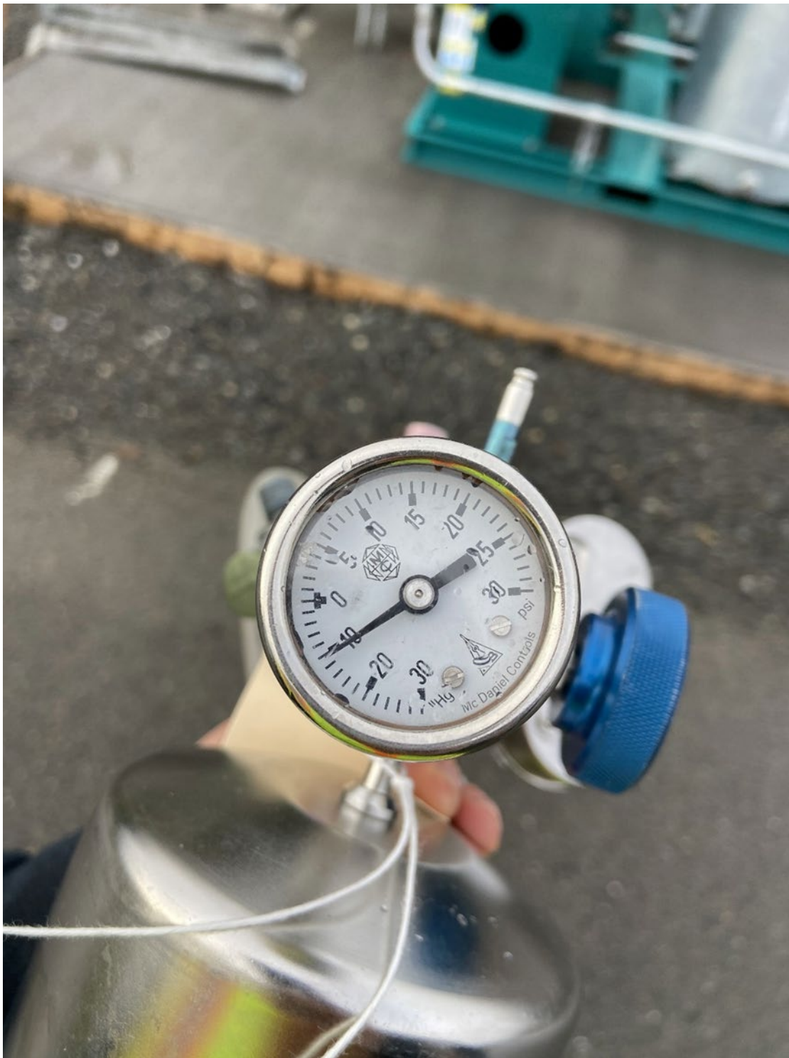
Figure 5. Pressure Gauge for North Blower Sample with Final Vacuum of 10 Inches of Mercury
