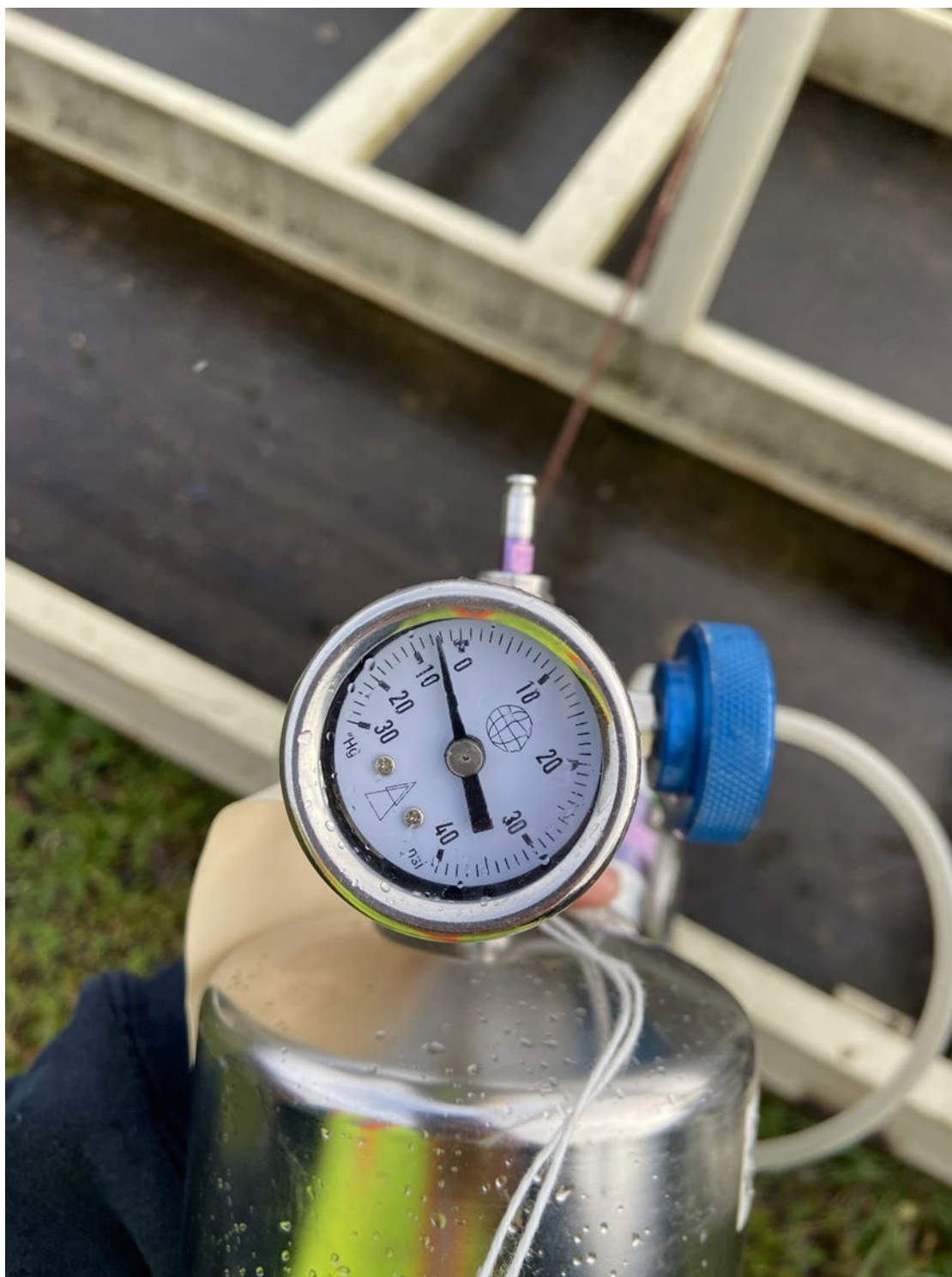
Figure 3. Pressure Gauge for South Blower Sample with Final Vacuum of 5 Inches of Mercury.
