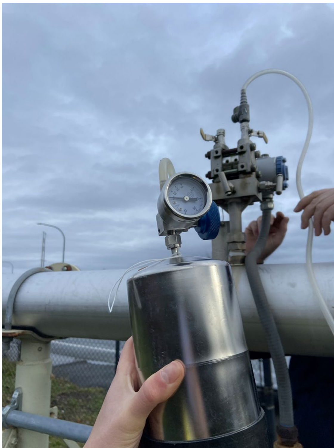
Figure 2. Pressure Gauge for South Blower Sample with Initial Vacuum of 30 Inches of Mercury.
