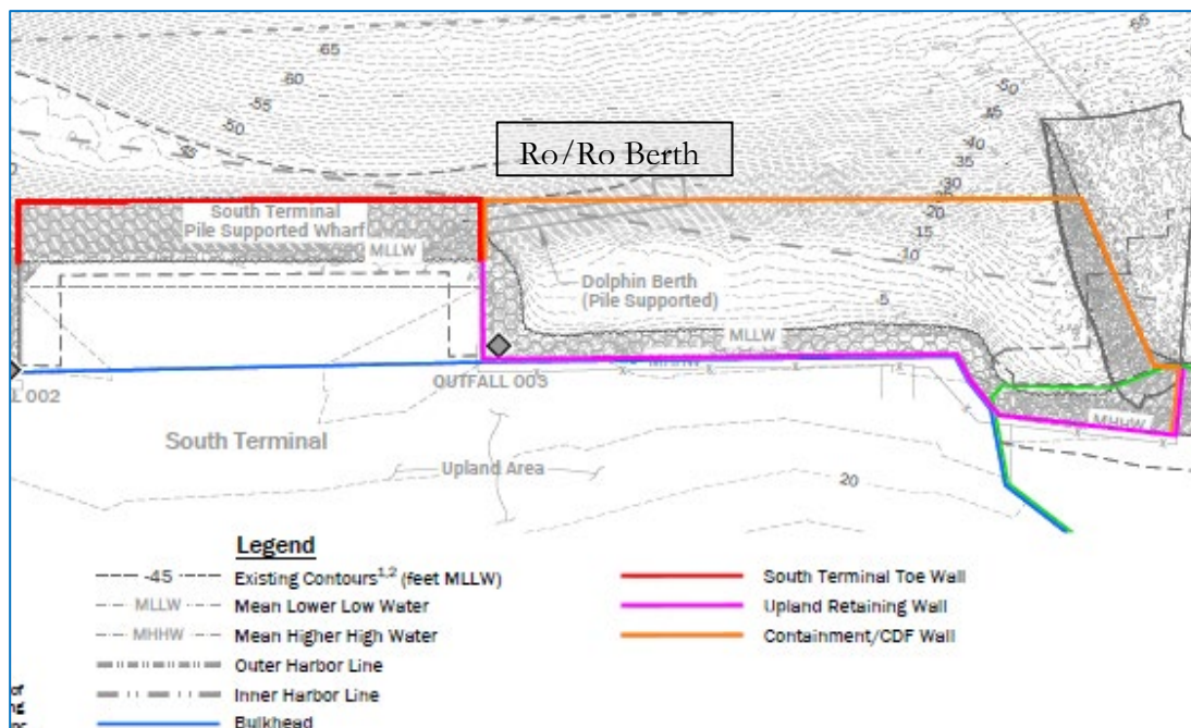
Figure 2 – Remedial Structural Element Layout
