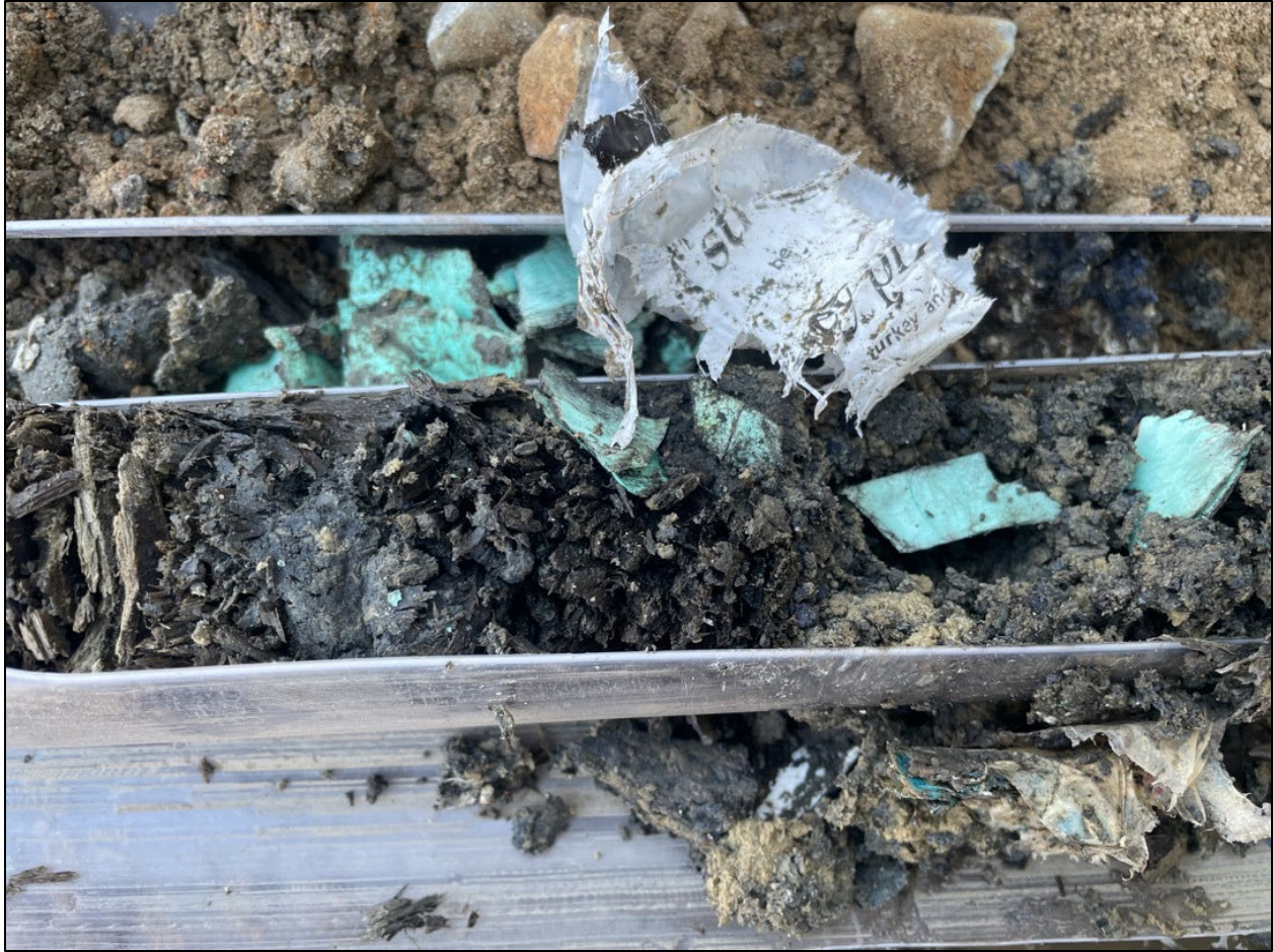
Figure 5 Typical landfill material (including plastic and Styrofoam) as observed within B-05.
