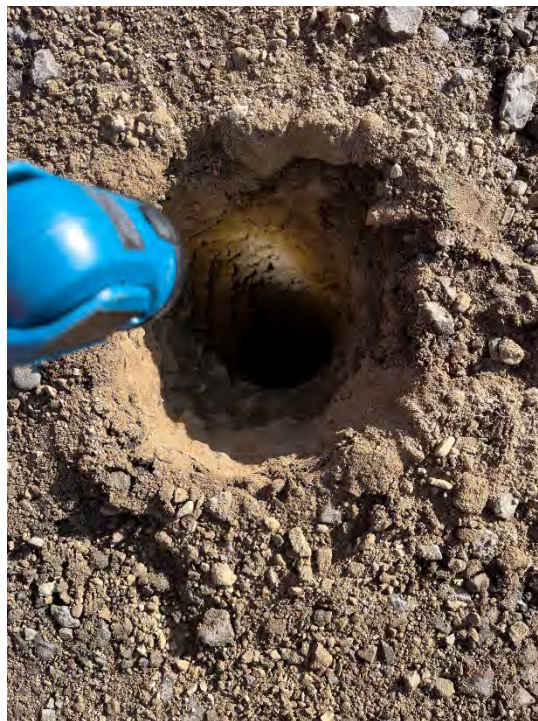
Photograph 10. Side-stepped past concrete (B-12).
