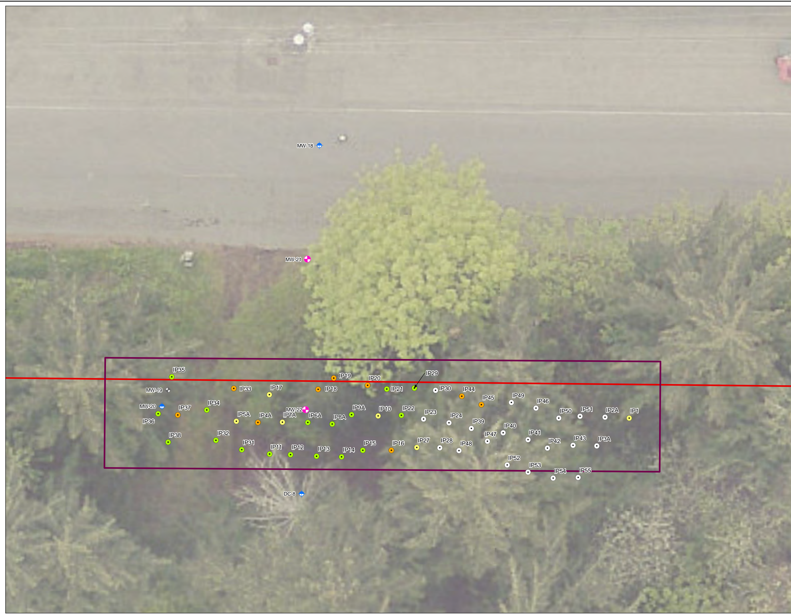
FIGURE 6 PRB LAYOUT AND WELL LOCATIONS MANHATTAN VILLAGE SHOPPING CENTER AND HARRIS PROPERTIES 17847, 17855 & 17817 FIRST AVENUE SOUTH NORMANDY PARK, WASHINGTON FARALLON PN: 578-002
