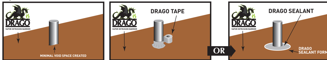
Fig. 4a: PIPE PENETRATION SEALING
