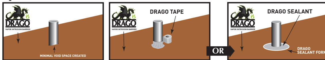
Fig. 4a: PIPE PENETRATION SEALING
