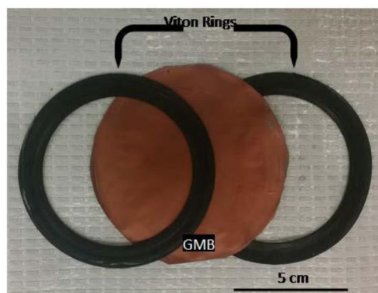
Figure 2: Membrane and Viton Rings
