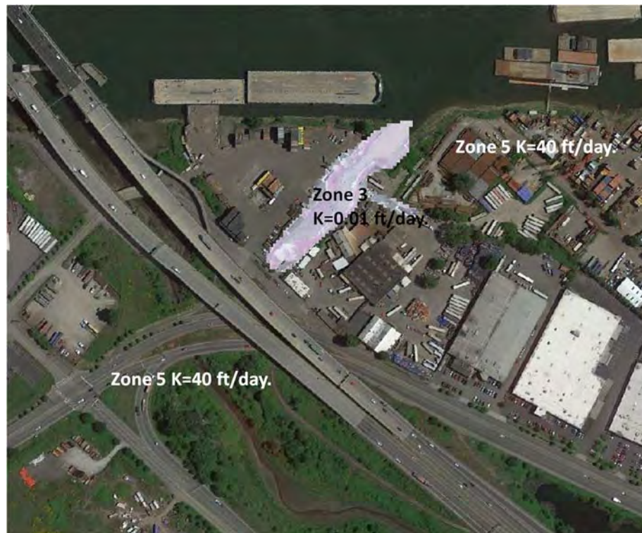
Figure 8. Horizontal hydraulic conductivity zones in model Layer3.
