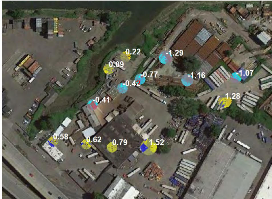
Figure 12. Water level residuals (ft) for the upper sand unit (model layers 1 and 2). Yellow denotes locations where model values are greater than observations; blue denotes locations where model values are less than observations.
