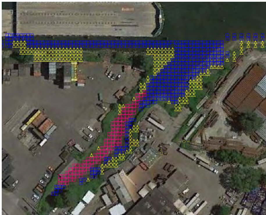
Figure 9. Location of cemented area in model Layer 1. Red symbols denote locations along the Embayment boundary with cemented conditions. Blue symbols denote areas without cemented conditions. Yellow symbols denote drains.
