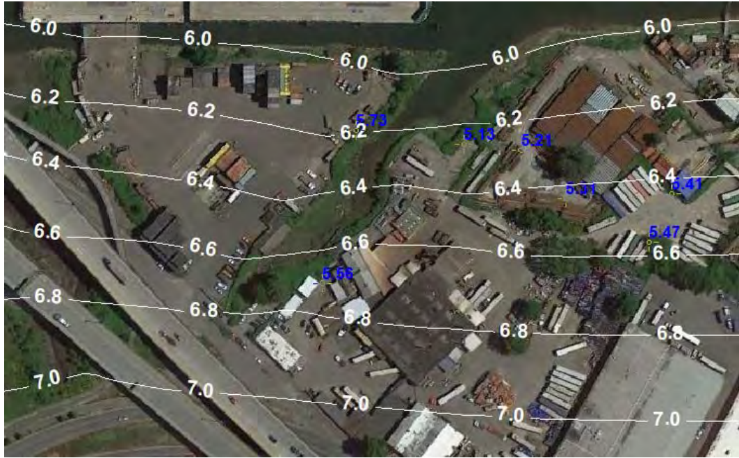
Figure 16. Model water level contours for the lower sand unit (model Layer 4)
