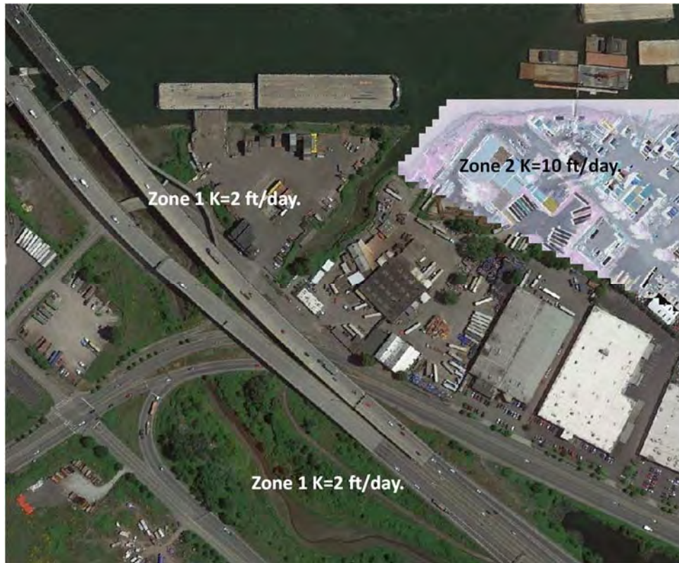
Figure 6. Horizontal hydraulic conductivity zones in model Layer 1.
