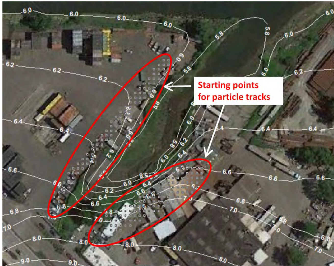
Figure 4. Modeled average water level contours in the upper sand zone for the current-conditions scenario and starting locations for particles used to depict groundwater flow pathways.
