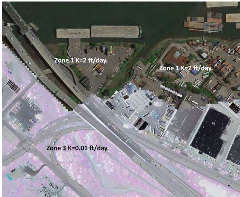
Figure 7. Horizontal hydraulic conductivity zones in model Layer 2.
