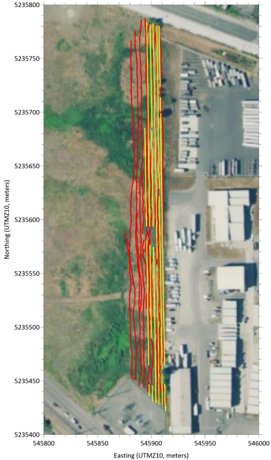
Figure 3. Geophysical survey coverage for GPR (Red) and EM (Yellow) survey lines.
