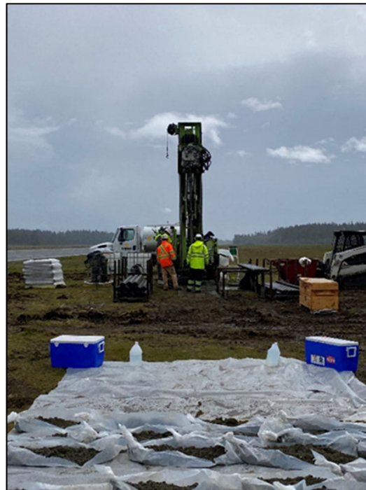
Drilling new monitoring well and soil samples
