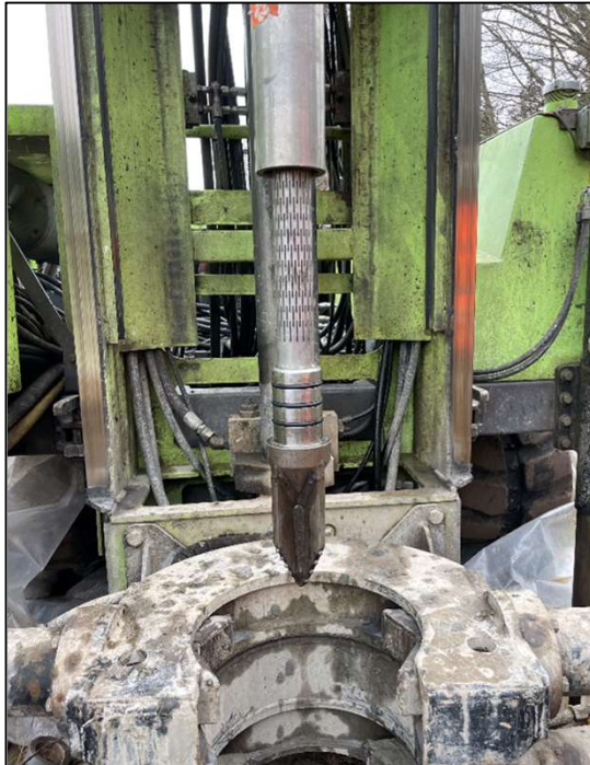
Sampling tool used to obtain groundwater samples
