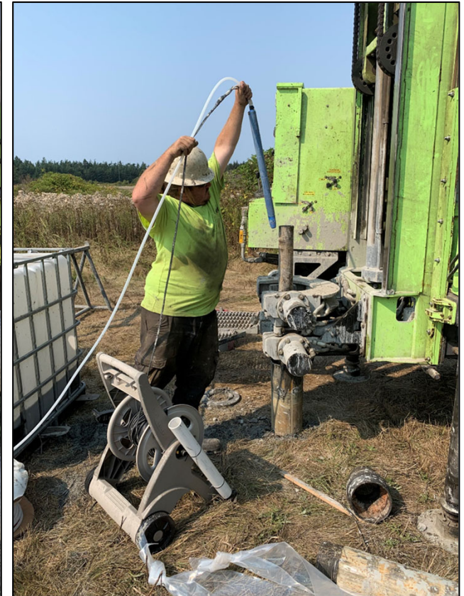
Discrete groundwater sample collection at Current Fire Training Area
