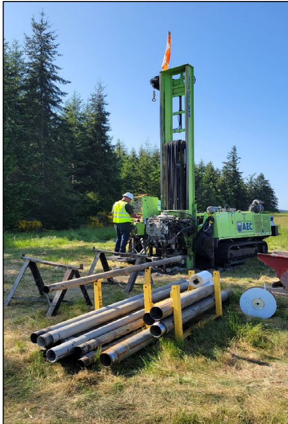
Drilling new monitoring well and collected soil samples at OLF Coupeville
