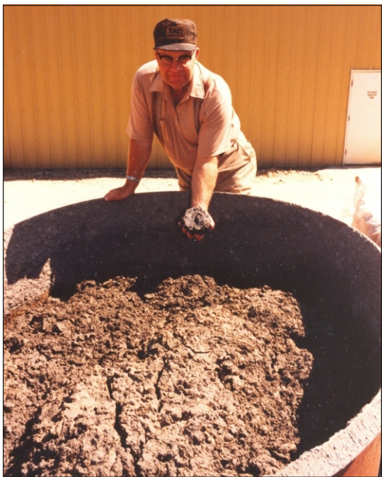
Figure 16. Madre silver-lead-zinc concentrate ready for shipment to the Cominco smelter at Trail, B.C., October 1983. Brownish cast of concentrate is due to high sphalerite content. (Photo courtesy of Mack M. Slate.)
