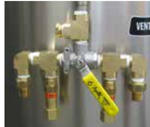
Dual Safeties & Rupture Discs— Diverter valve allows to safely change relief valves or rupture discs without depressurizing the tank. (Optional on all models / standard on Perma-Cyl horizontal, 5500, 2000 CO 2 HP & FlexFill)
