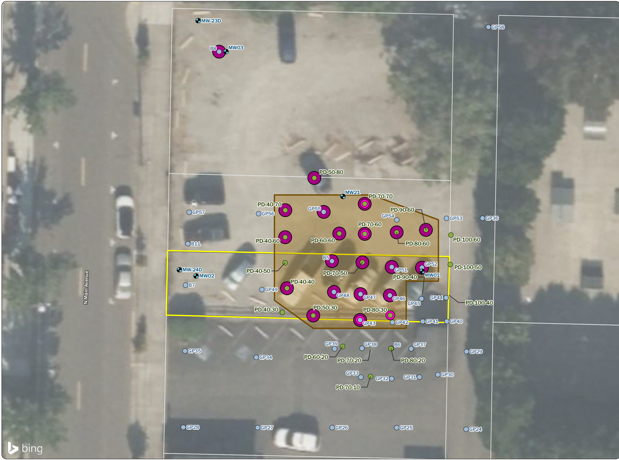
Figure 2-4 Deep Soil Excavation Area (up to 14.5 feet bgs)
