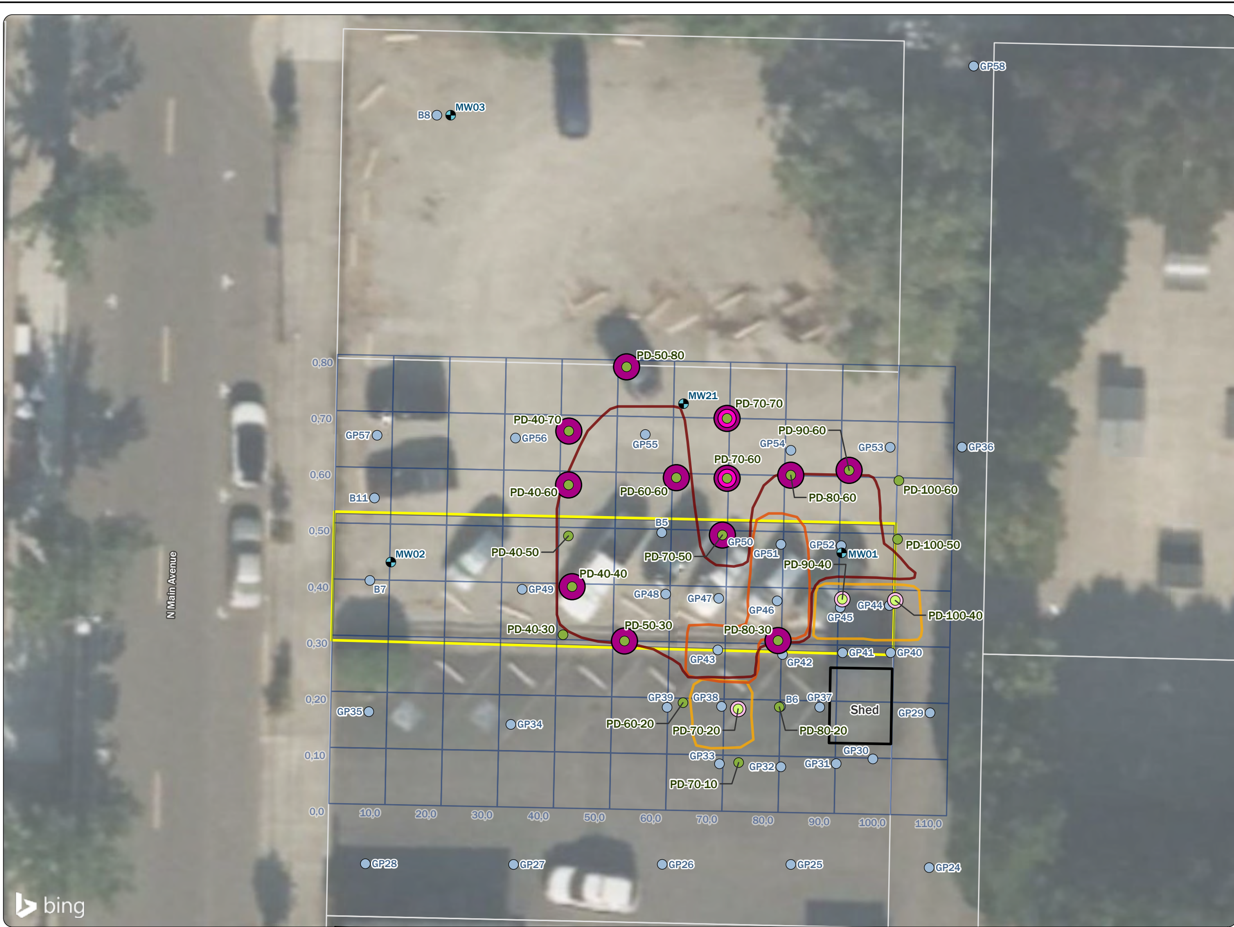
Figure 3 Geoprobe Locations to Support Remedial Design in Source Area
