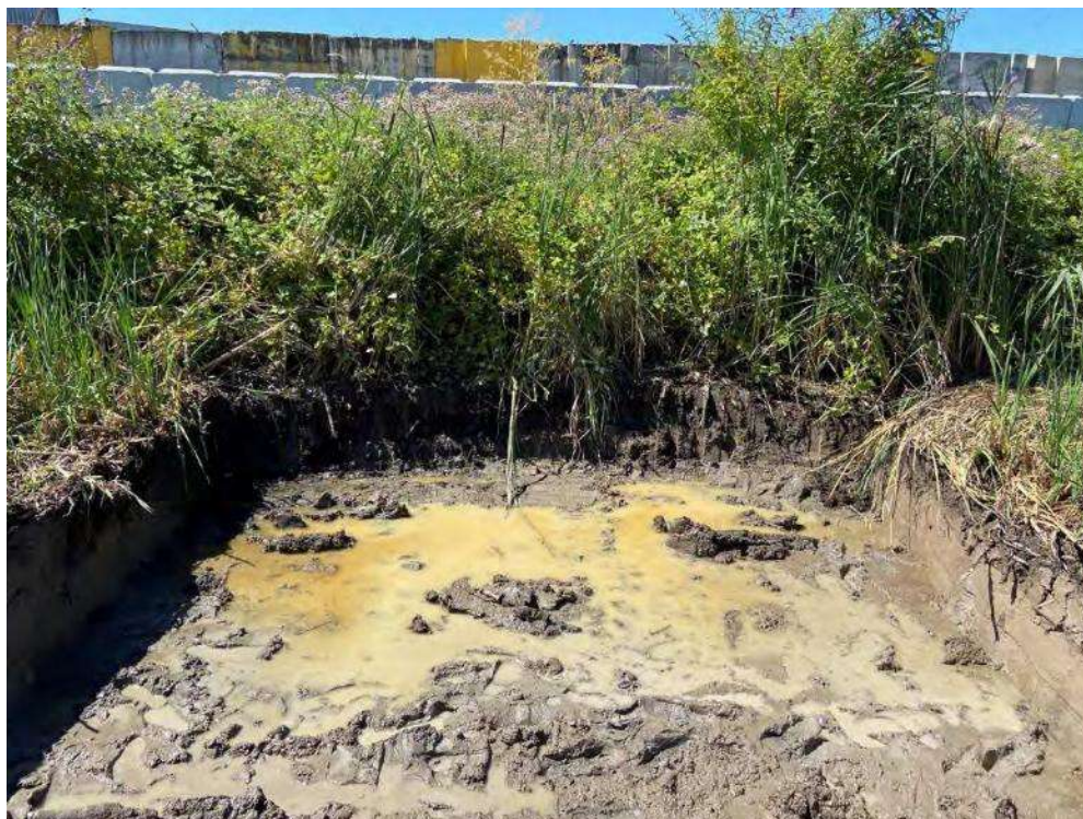
Figure 39: Bottom of RAU D1 NOTE: Clay-rich Silt bottom
