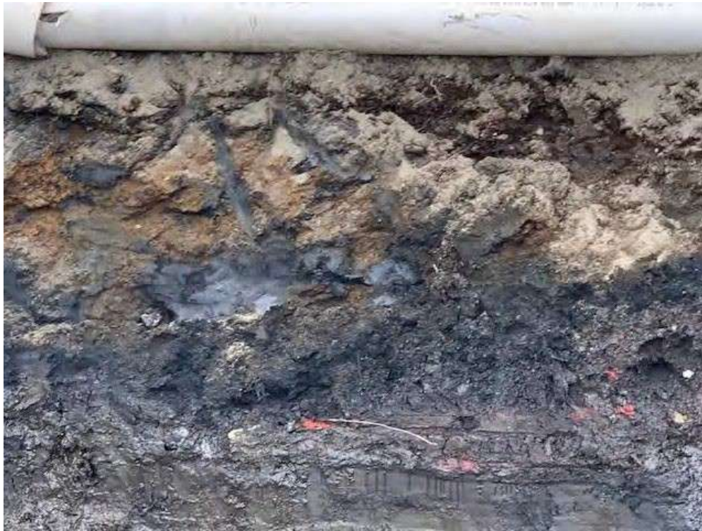
Figure 25: RAU B5: Close up Eastern sidewall at 0-5 feet – NOTE: Presence of “Shot” in center of photograph
