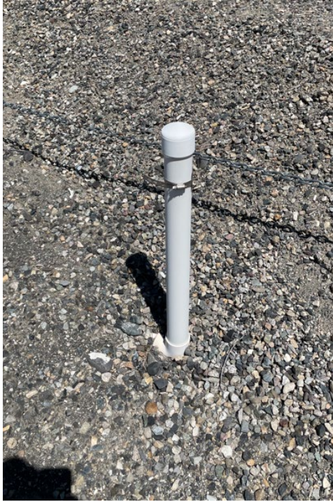
Well AR-07. No protection
