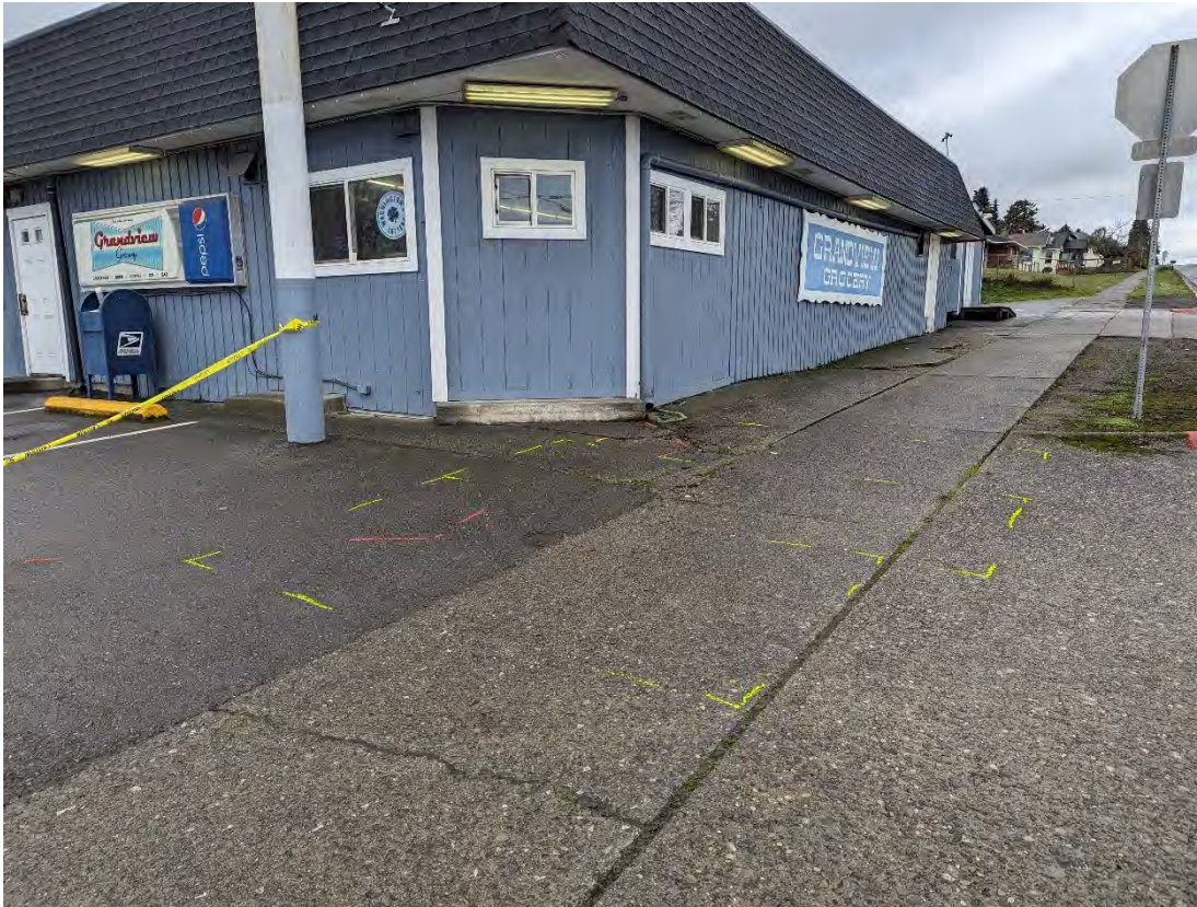
View of three anomalies (suspected USTs) near the northeast corner of the convenience store, looking westward. Each anomaly is identified with yellow paint.
