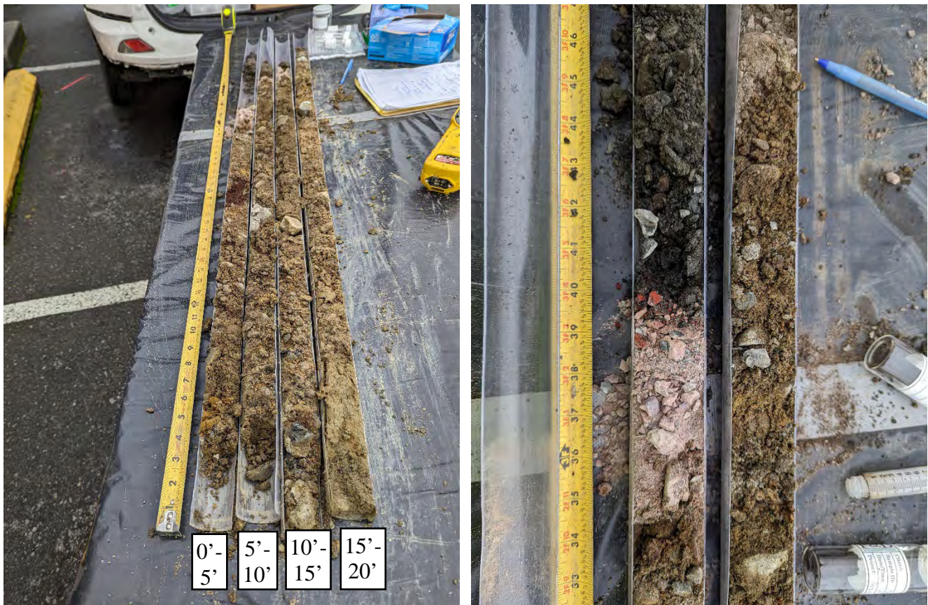
Soil cores from B4. Close up of soil core in right side photo shows the dark colored contaminated soil (B4-1) on top of red/pink-dyed concrete.
