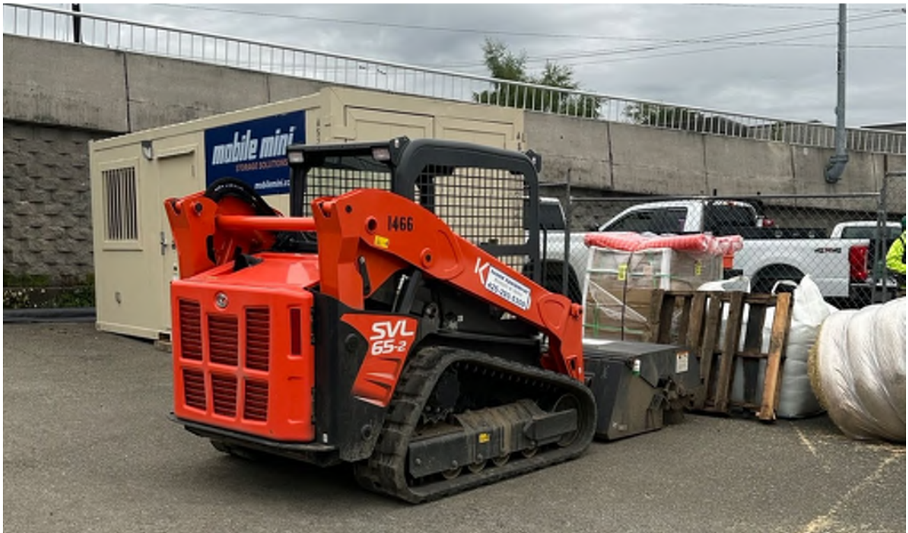
Photo 4. Kubota SVL65-2 Used for Sweeping Sediment on Site at the End of Each Shift.
