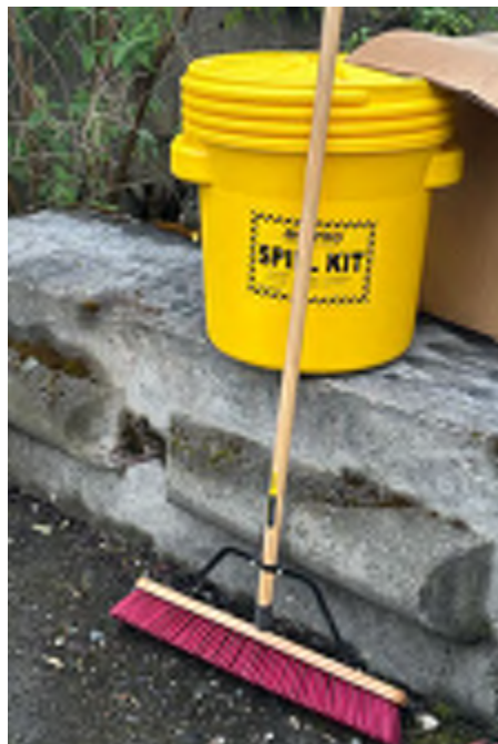
Photo 4. Spill Kit with Broom for Sweeping Sediment Off Roads.
