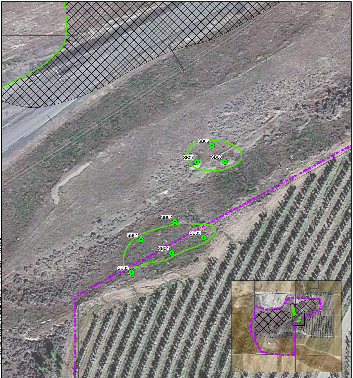
Figure A2-1 Proposed Boring Locations: Former Septage Lagoons
