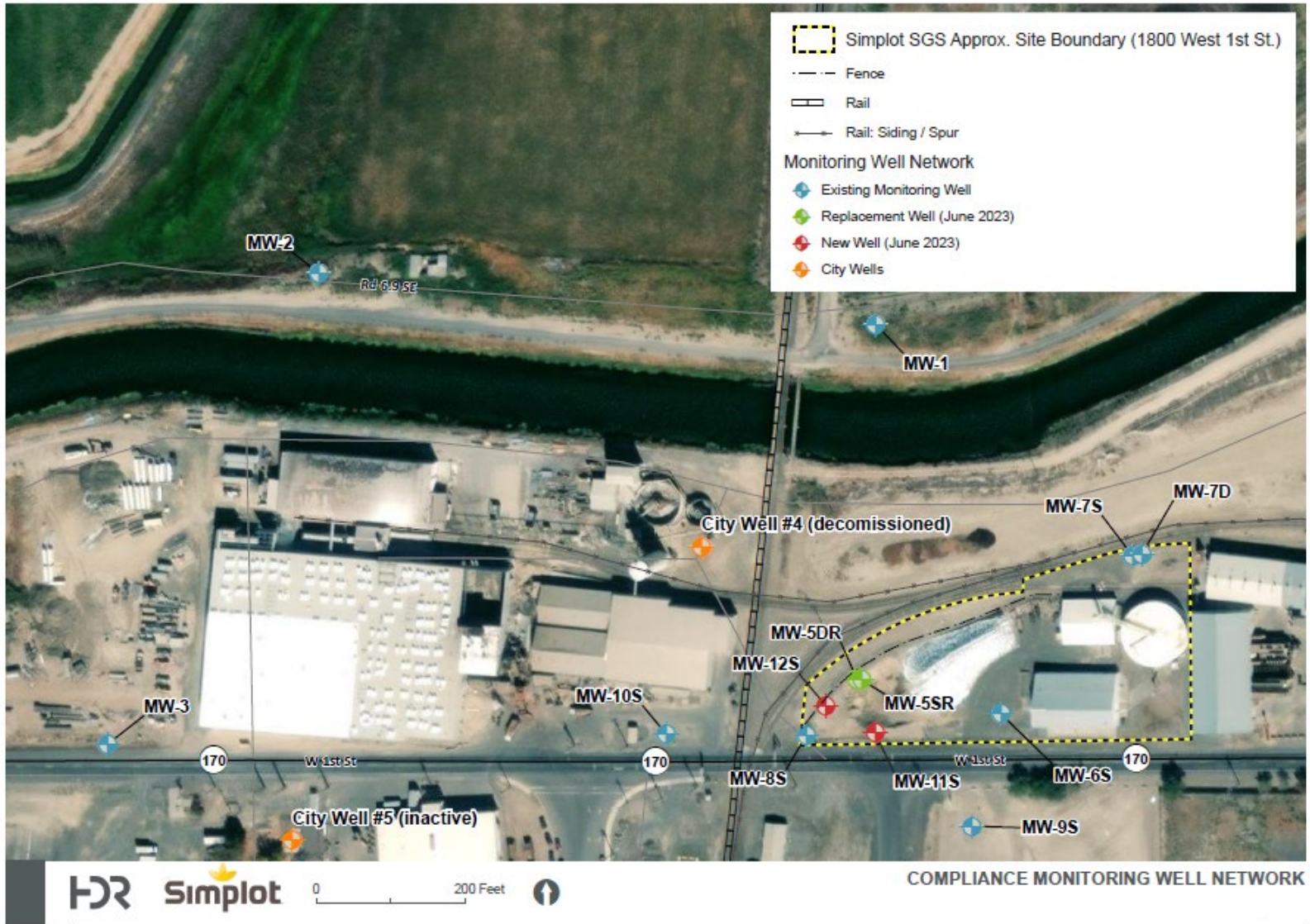
Figure 3, Existing Groundwater Monitoring Wells from HDR (October 2023)
