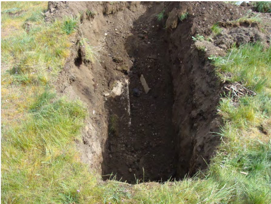
Test Pit 2 – Small amount of glass debris & concrete slab uncovered (<5% debris).
