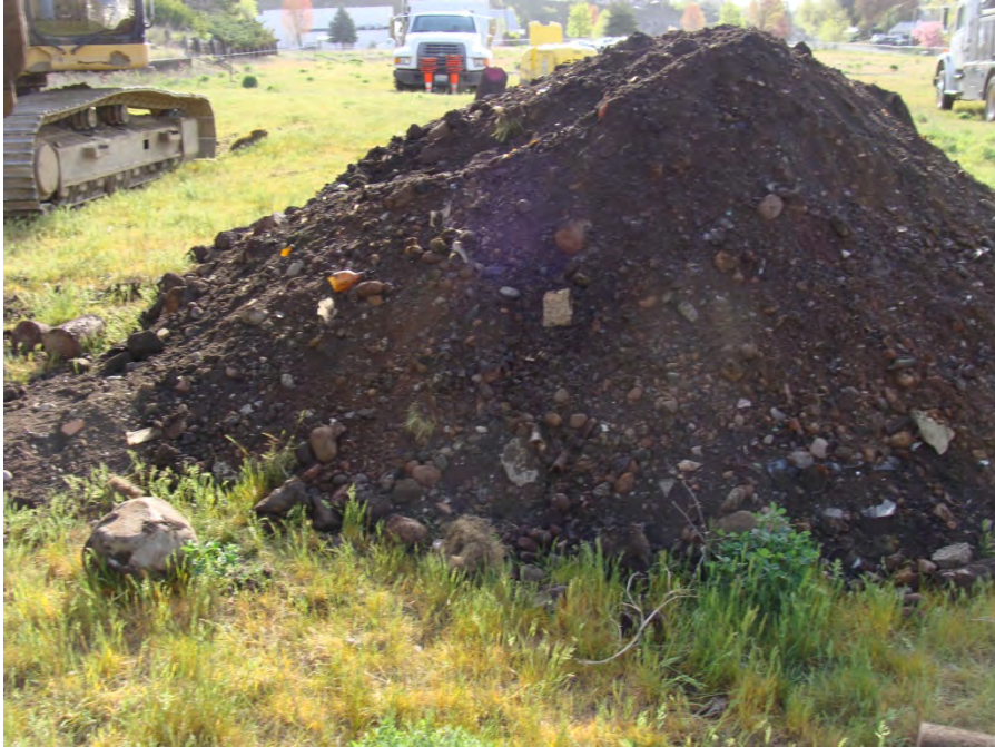
Test Pit 1 – Significant glass, porcelain, and metal debris excavated from pit (30% debris).
