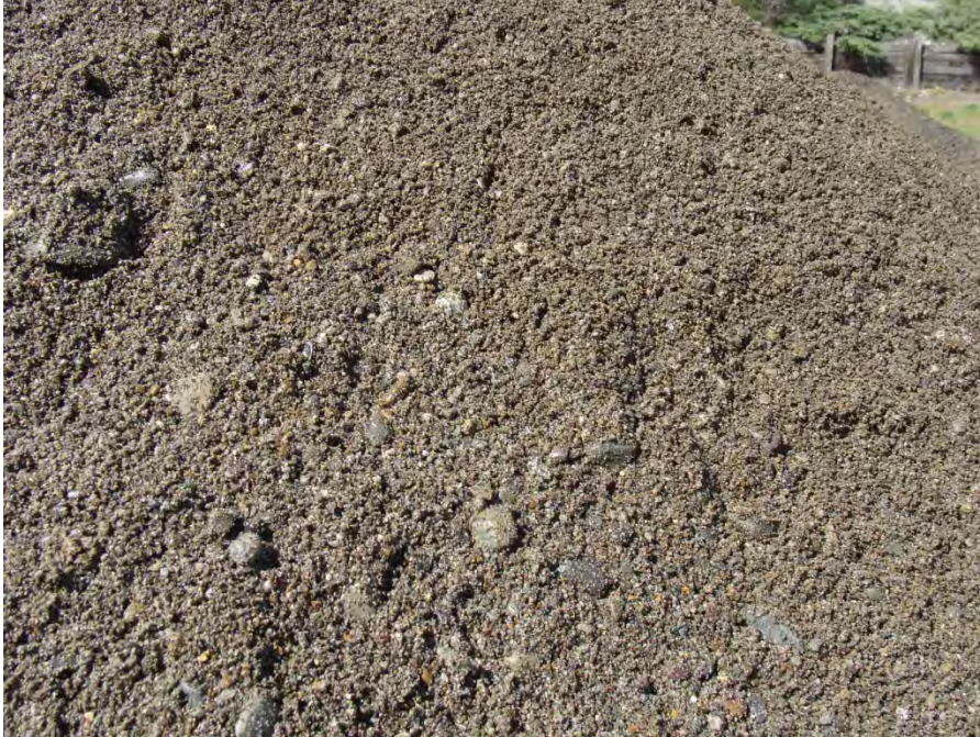
Test Pit 7 – Gravel with sand fill material; trace debris found (<5%) .
