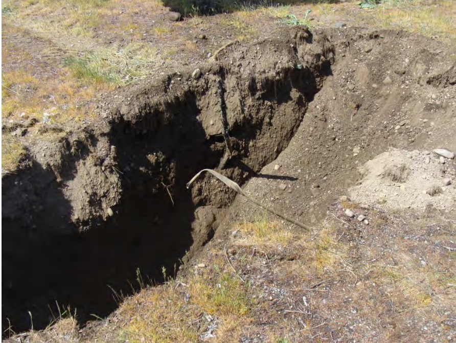
Test Pit 5 – Metal conduit found near-surface (<5% debris).
