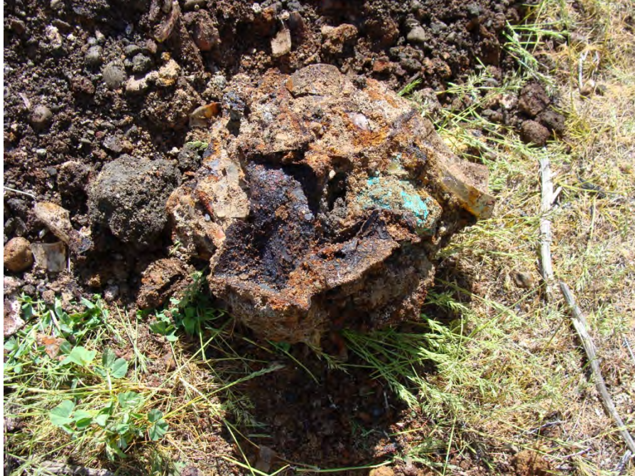
Test Pit 3 – Significant debris including cinder and slag-like material, glass, spoon, metal and porcelain (10-15% debris).
