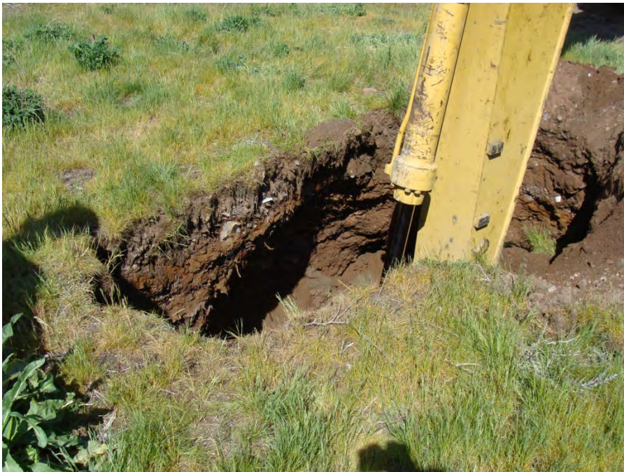
Test Pit 8 – Significant debris fill observed near the surface (15% debris).
