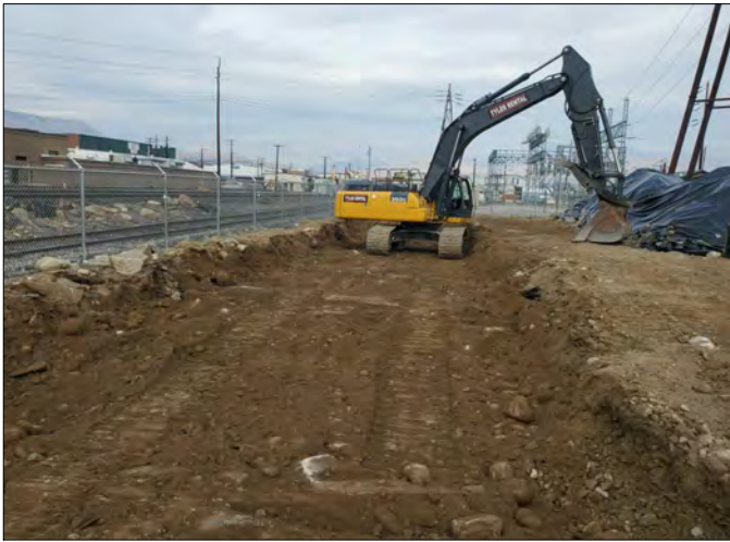
PHOTO 4 John Deere 350 Tracked Excavator.
