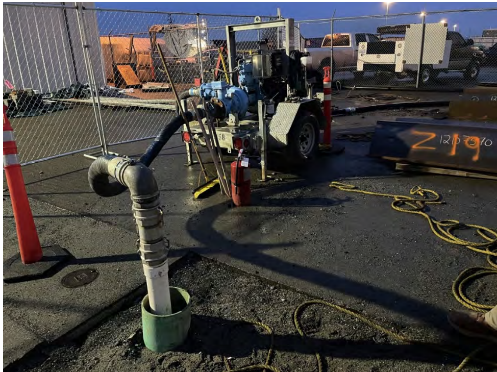
Photo 1. Pump located on northwest corner of site that requires installation of a secondary containment system.
