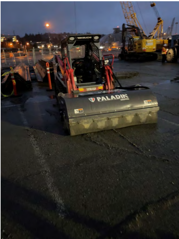
Photo 2. Site sweeper attachment for asphalt cleaning.
