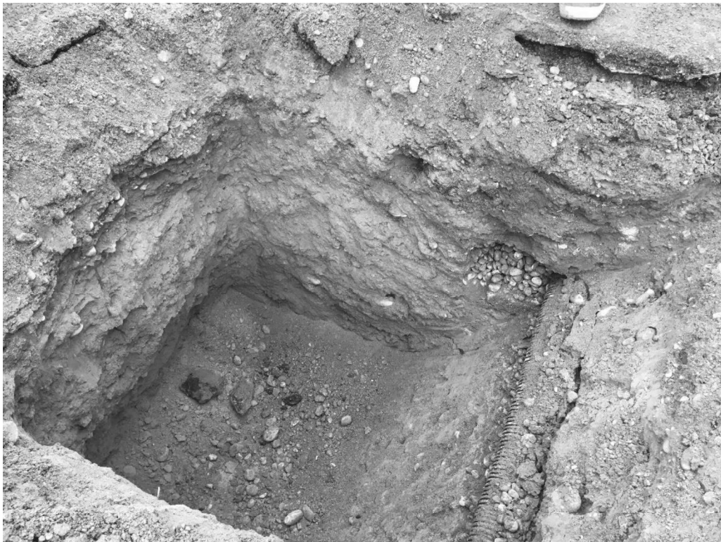
Photograph 2: Drain field test pit PH232-3, showing fill soils, piping, and native soil
