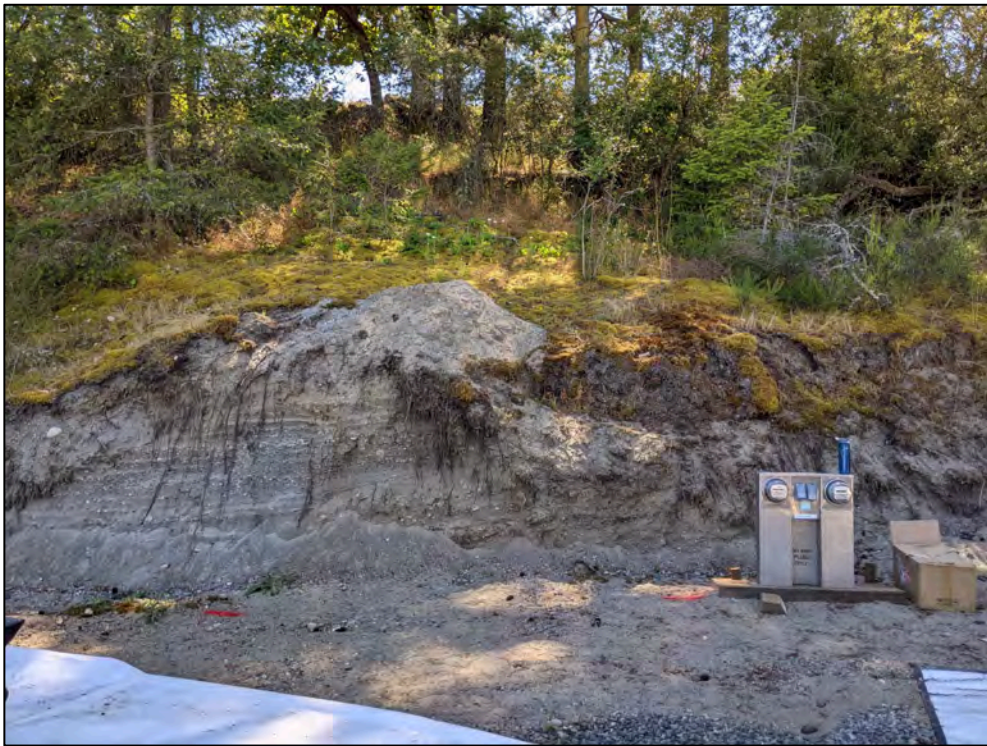
Figure 9. Typical glacial deposits exposed in the southwestern edge of the project, view to the south.
