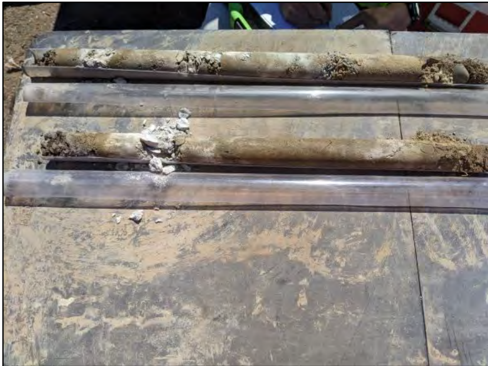
Figure 14. Representative image of bores encountering topsoil above glacial sediments. Image of SRWA-12 bore materials, showing sediments from 0-5 ft bs.
