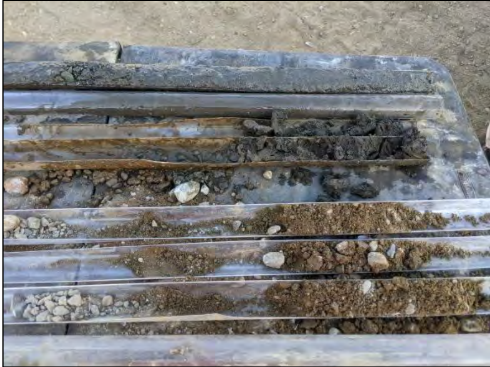
Figure 13. Representative image of bores encountering fill above beach. Image of BLWA-13 bore materials, with sediments from 0-5 ft bs present in the lower three tubes and 5-10 ft bs in the upper tubes.
