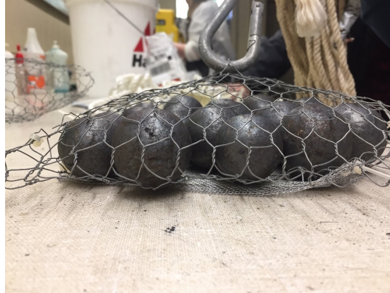
Photo 2. Side view of conceptual prototype with 1.5-2" steel balls secured in wire pouch.
