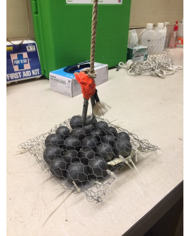
Photo 3. Top view of conceptual prototype with caribeenner attached to top of weighted bag with rope line.
