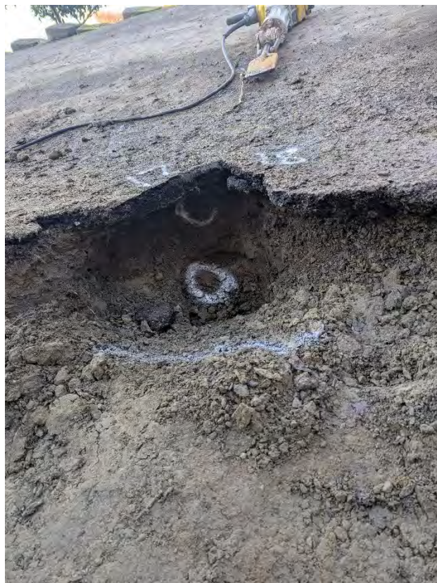
View of sample locations collected in sandy gravel fill beneath asphalt (sample 17) and below perforated pipe (sample 18).
