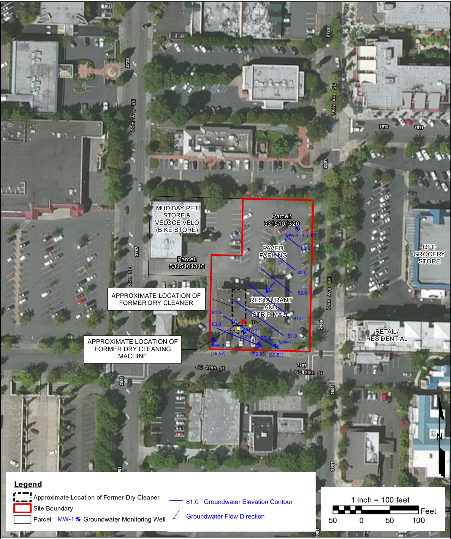
Figure 1 Site Plan with Sample Locations and Groundwater Elevation Contours
