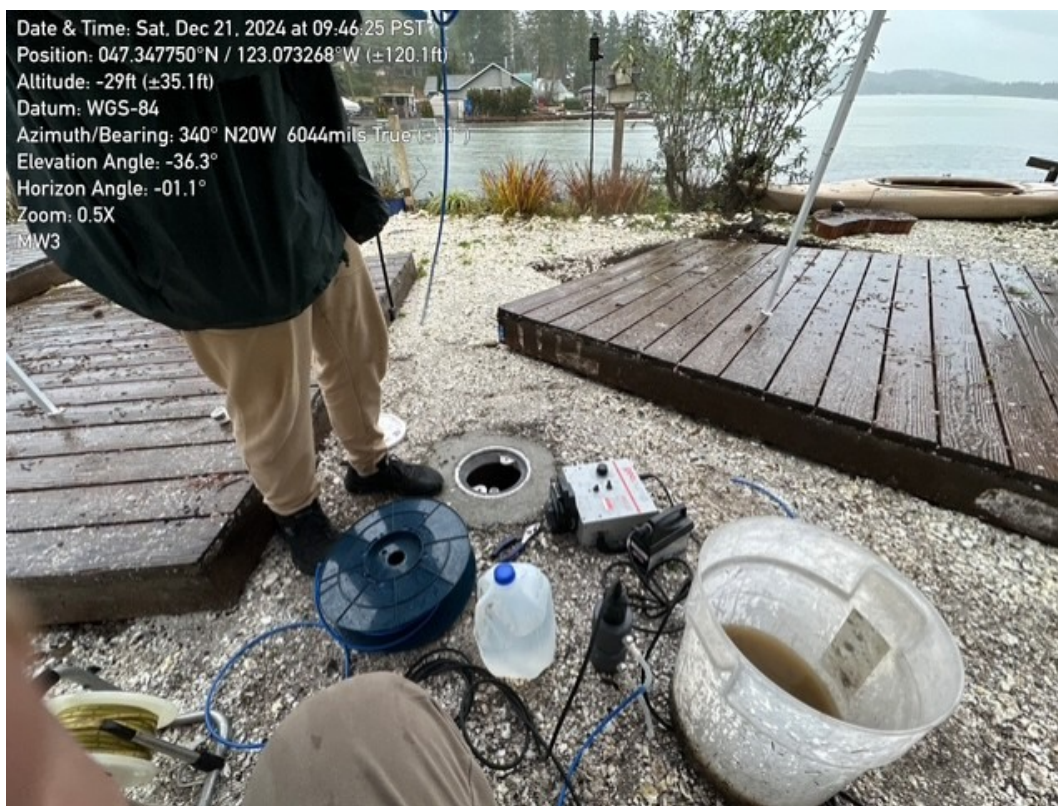
Photograph 4.10. View of typical groundwater sampling setup showing a peristaltic pump, discharge bucket, distilled rinse water and water chemistry meter.
