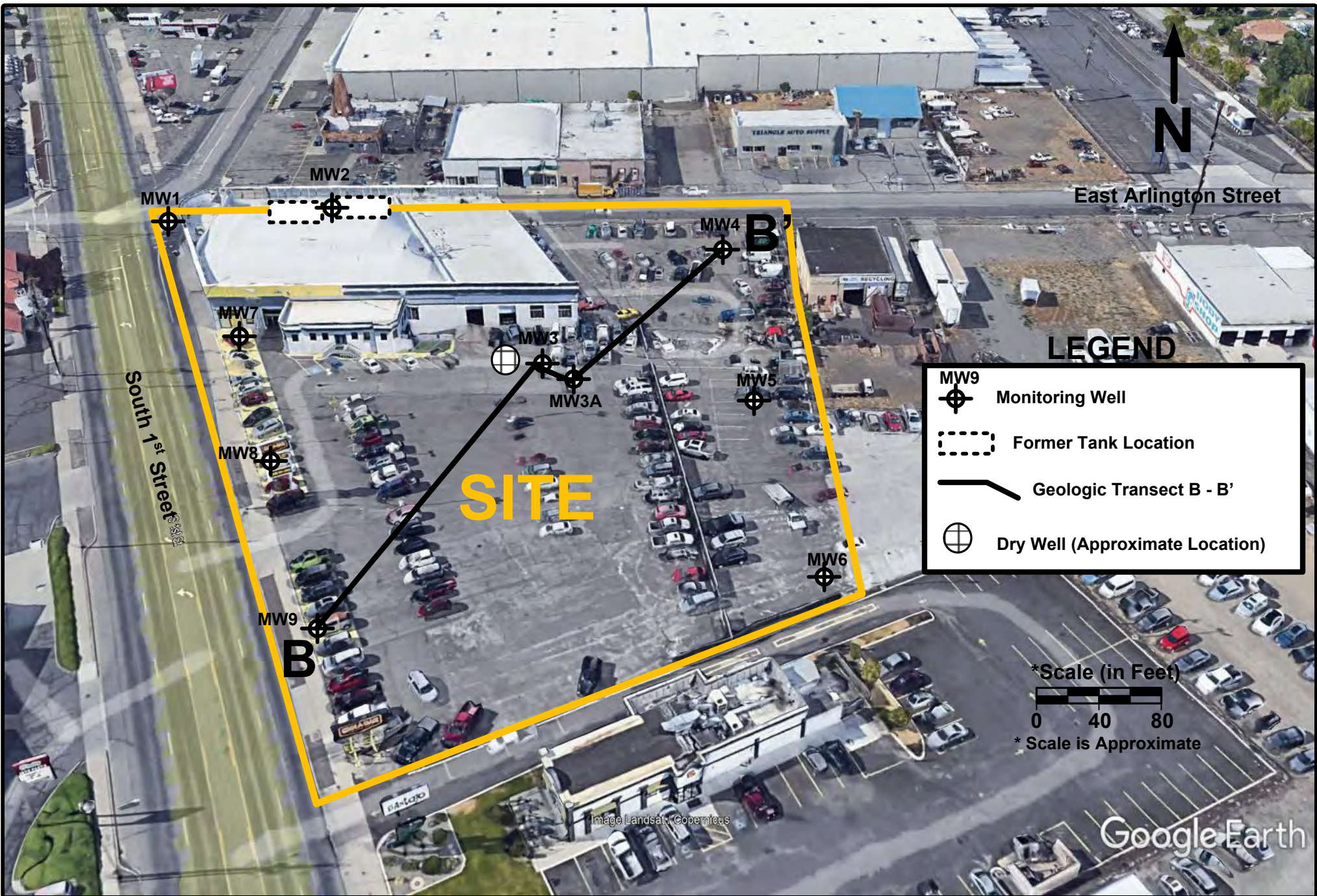
FIGURE 8 GEOLOGIC TRANSECT B - B'
