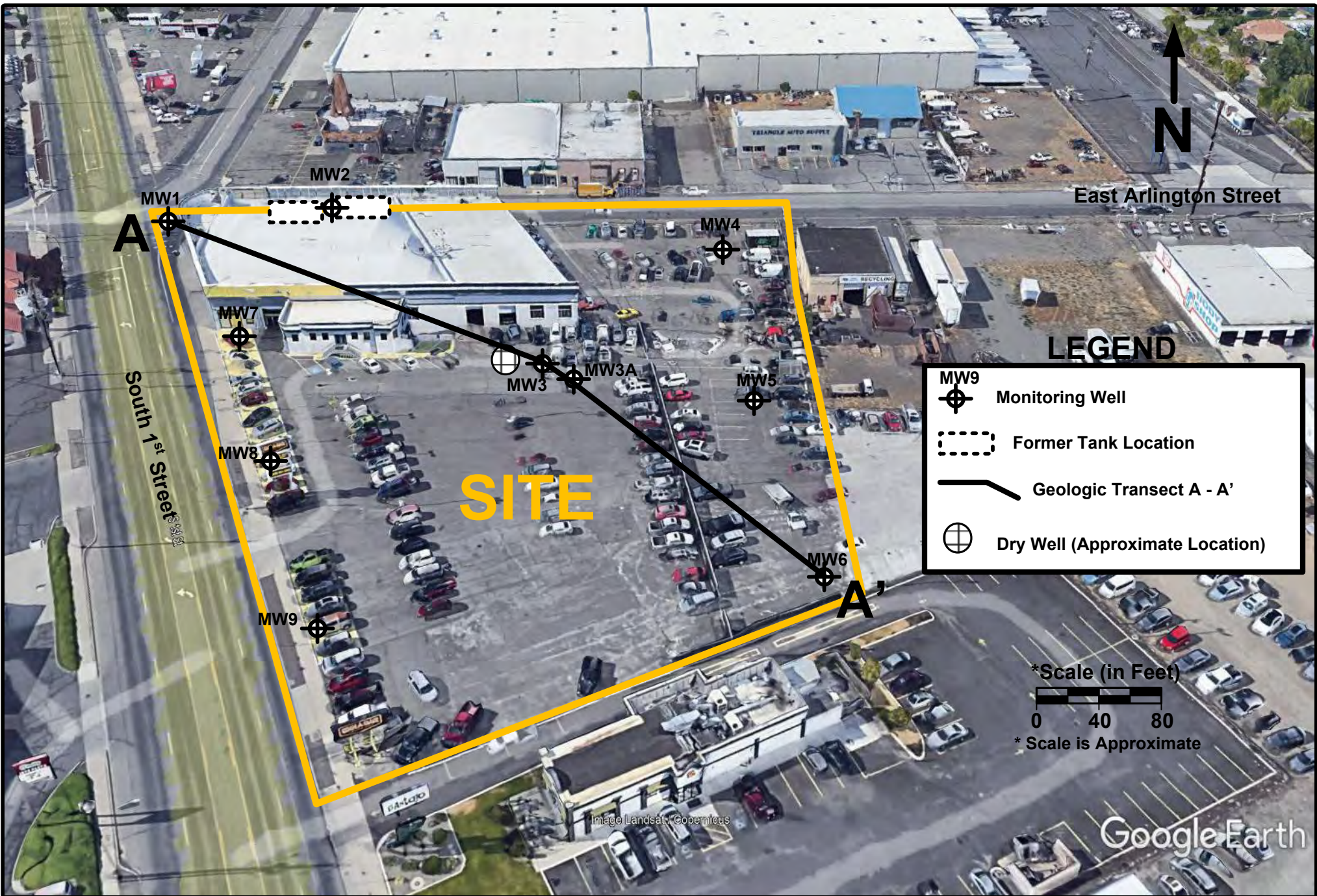
FIGURE 7 GEOLOGIC TRANSECT A - A'
