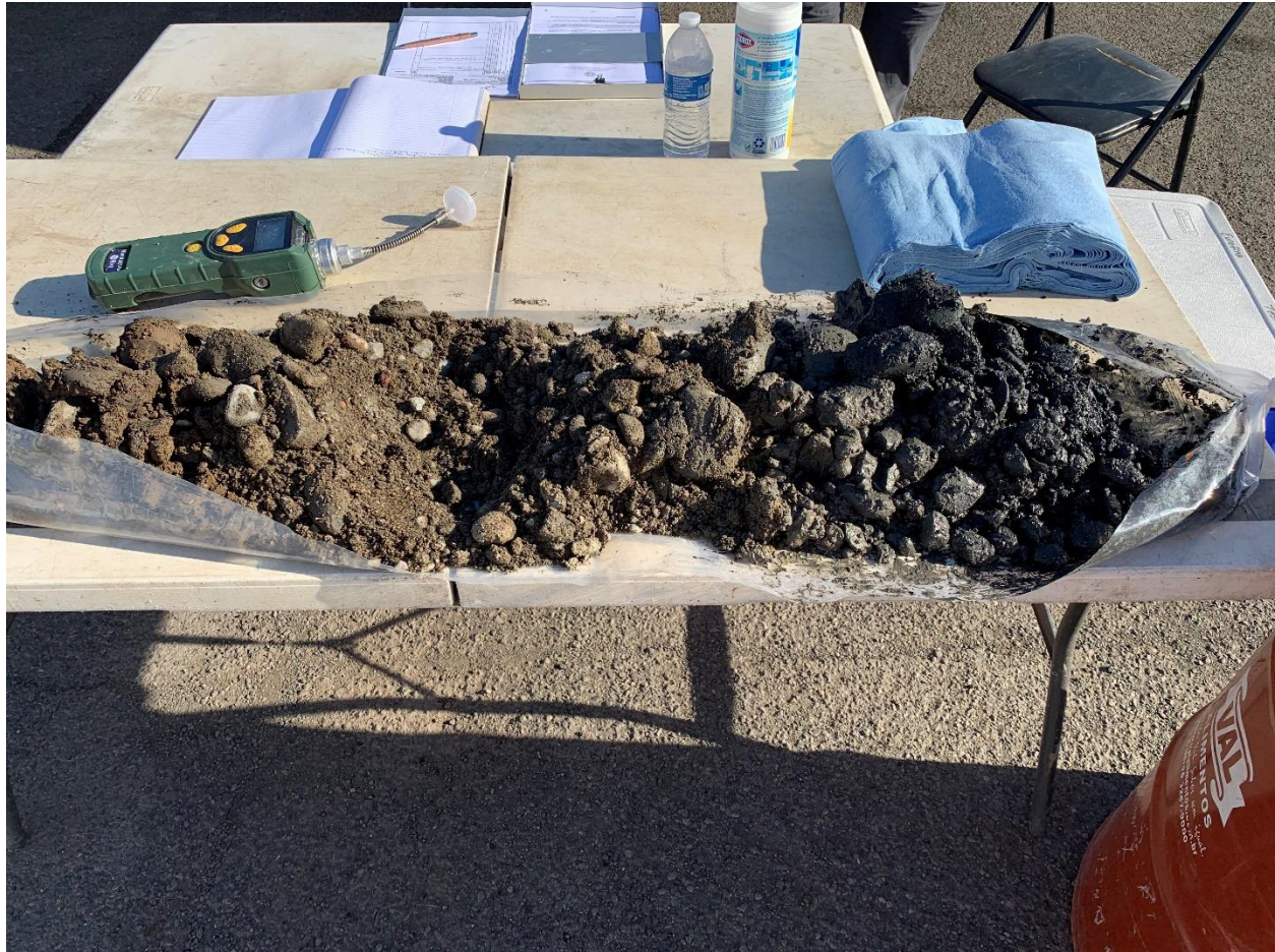
Photograph 8 – Soil lithology from 0 – 10 feet bgs in soil boring SB1. Note black, oil-stained soil from 7 – 10 feet bgs.
