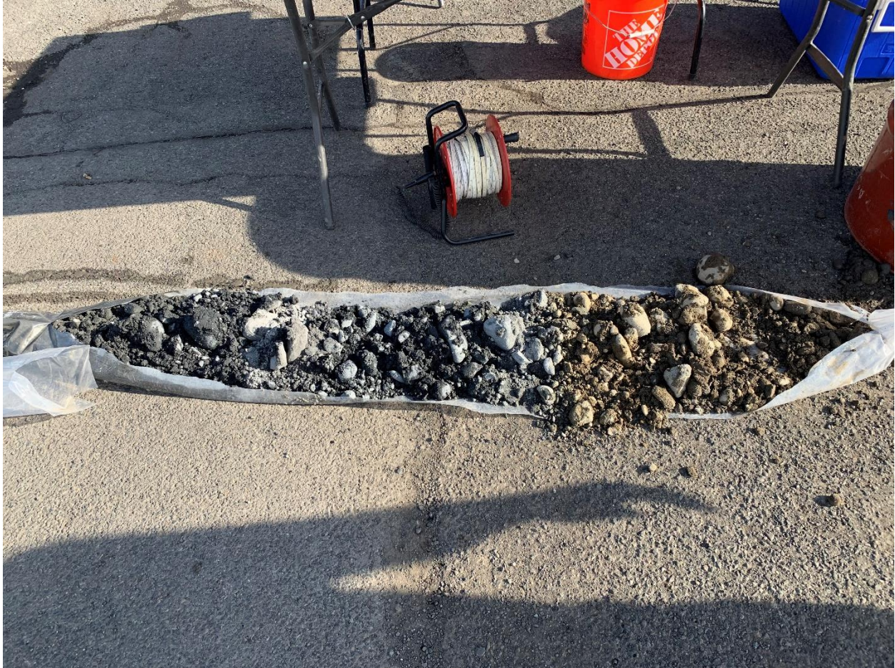
Photograph 9 – Soil lithology from 10 – 15 feet bgs in soil boring SB1. Note black, oil-stained soil from 10 – 14 feet bgs and relatively clean, brown soil from 14 – 15 feet bgs.
