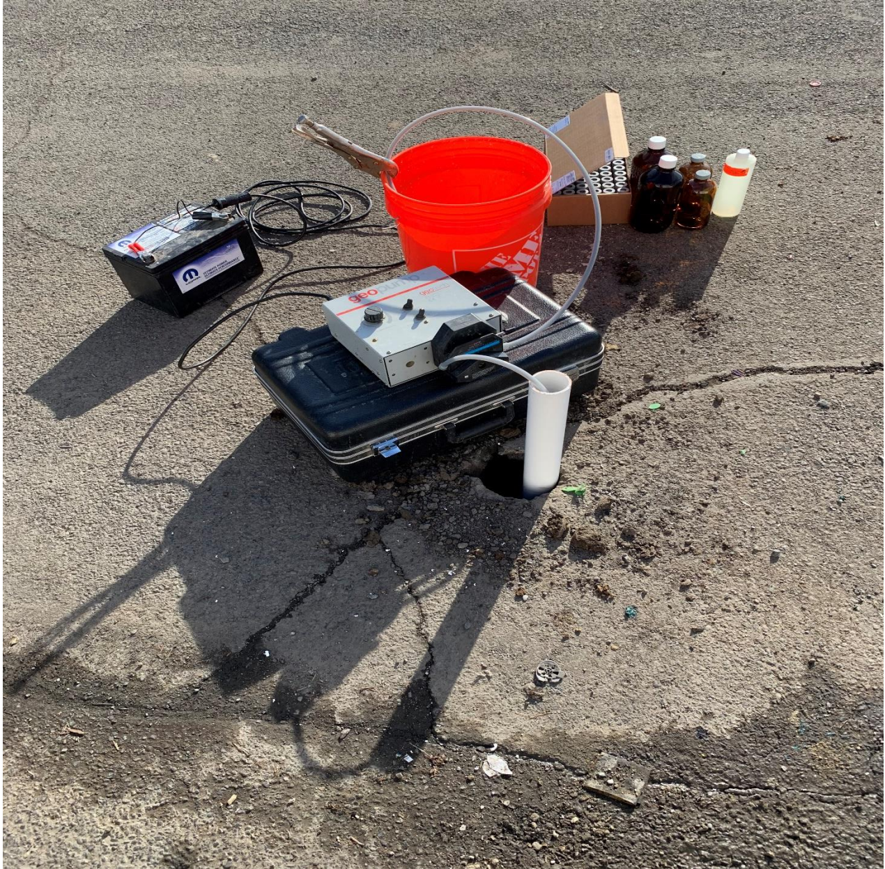
Photograph 10 – Groundwater sampling gear being utilized during the purging and collection of groundwater sample SB1-2-1-22-GW.
