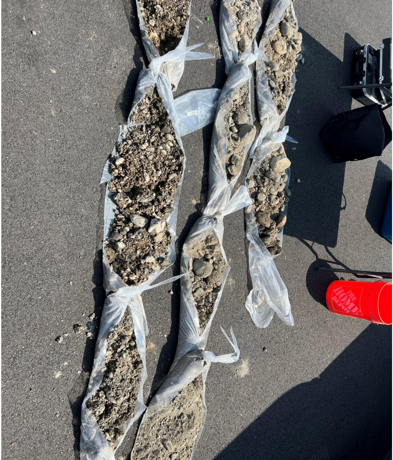
Photograph 4 – Soil cuttings from boring MW8 on May 19, 2023.
