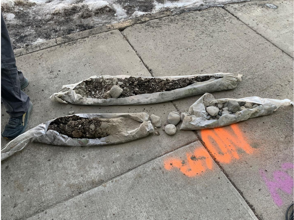
Photograph 14 – Soil lithology in soil boring SB4 from 0 – 10 feet bgs.
