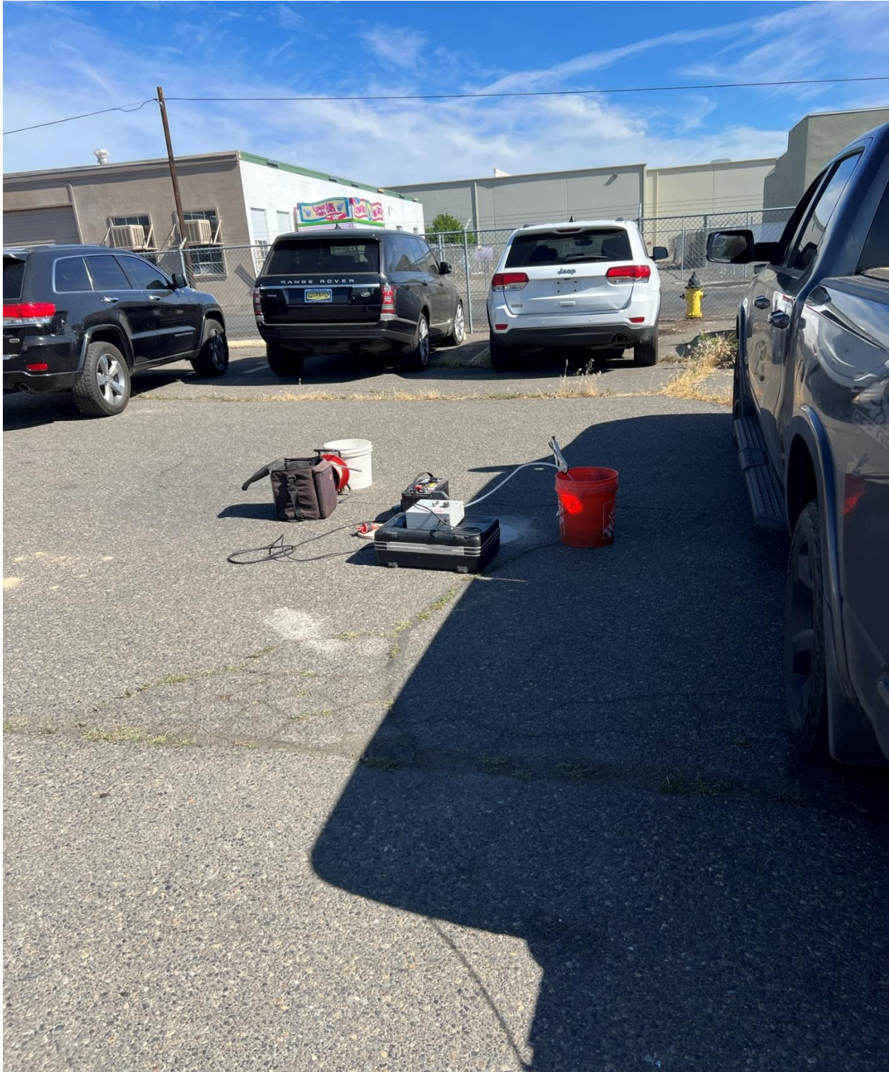
Photograph 10 – Purging groundwater from well MW4, prior to sample collection on June 13, 2023 (facing north).
