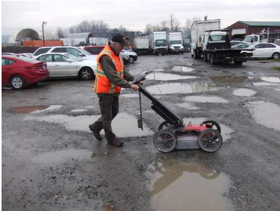
Photo 2. A view of the GPR survey.
