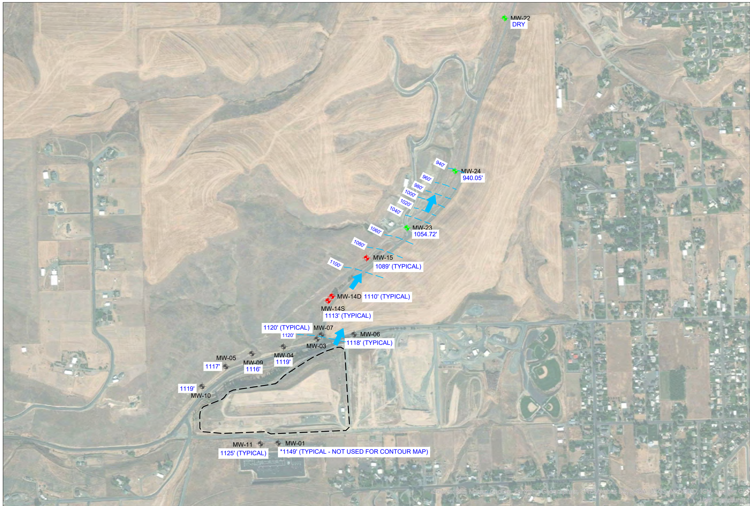
Figure 3. Groundwater Elevations and Flow Map
