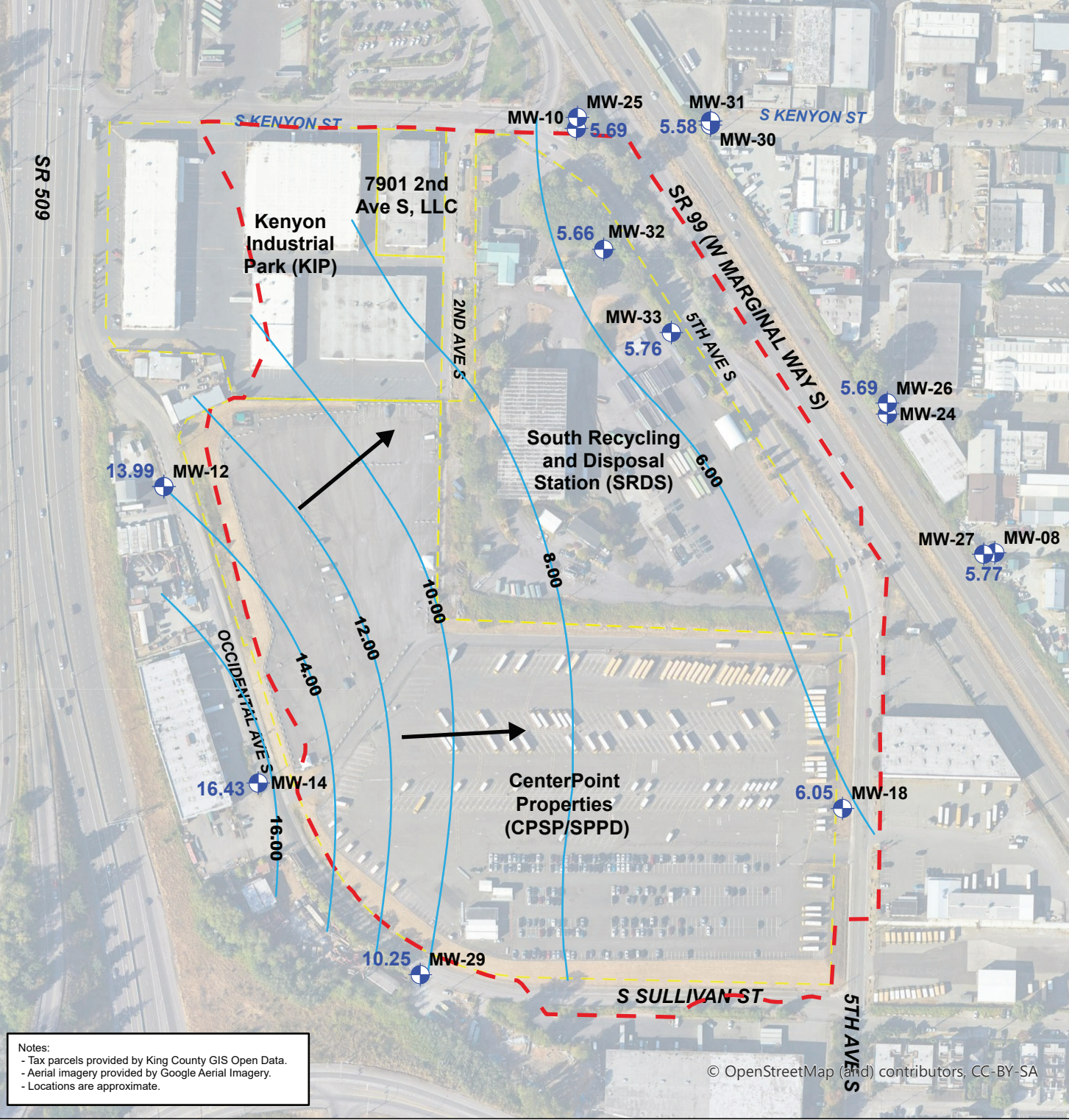
Figure 8 Potentiometric Surface Map August 6, 2024 South Park Landfill
