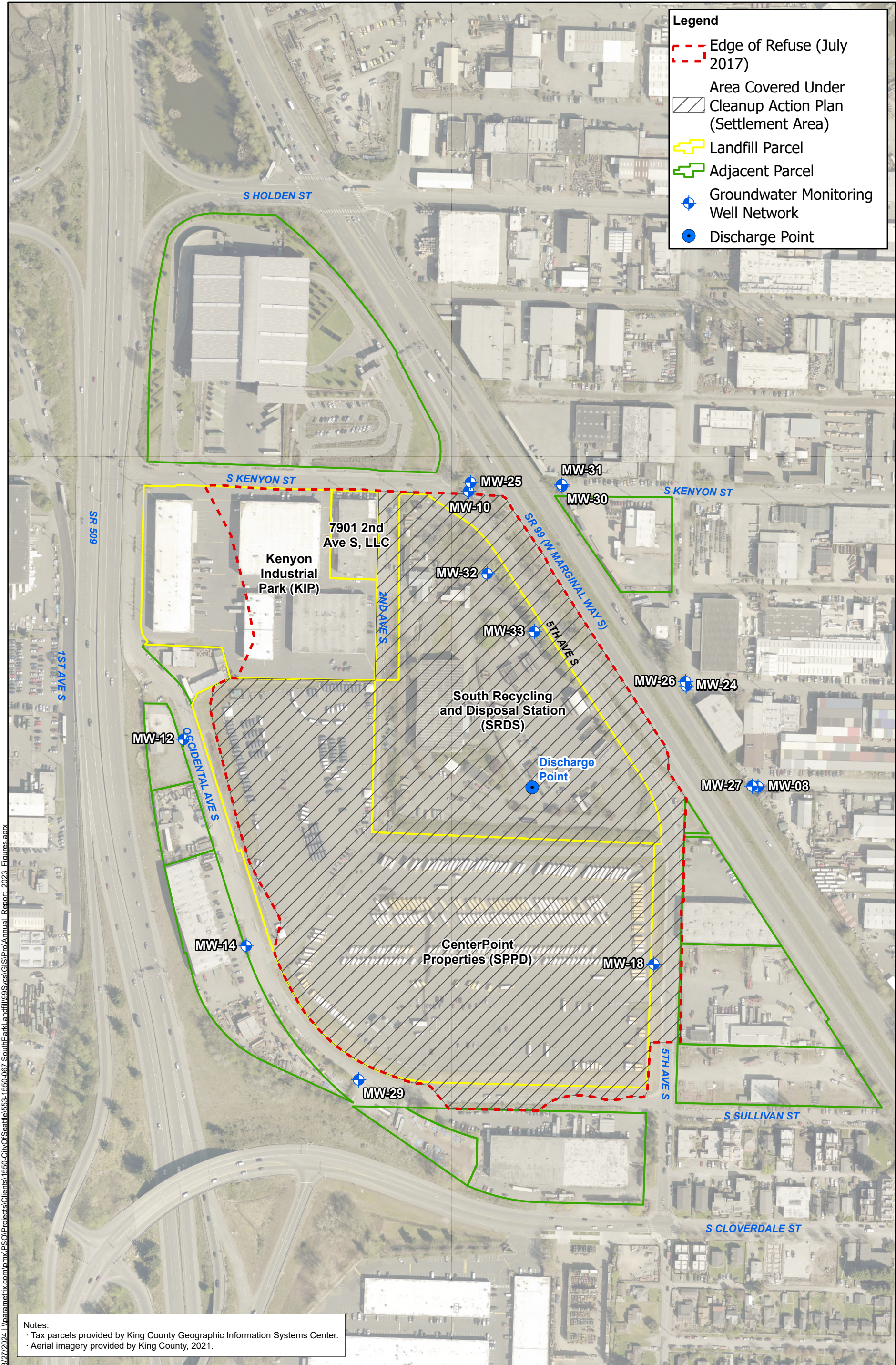
Figure 5 Groundwater Monitoring Well Network South Park Landfill
