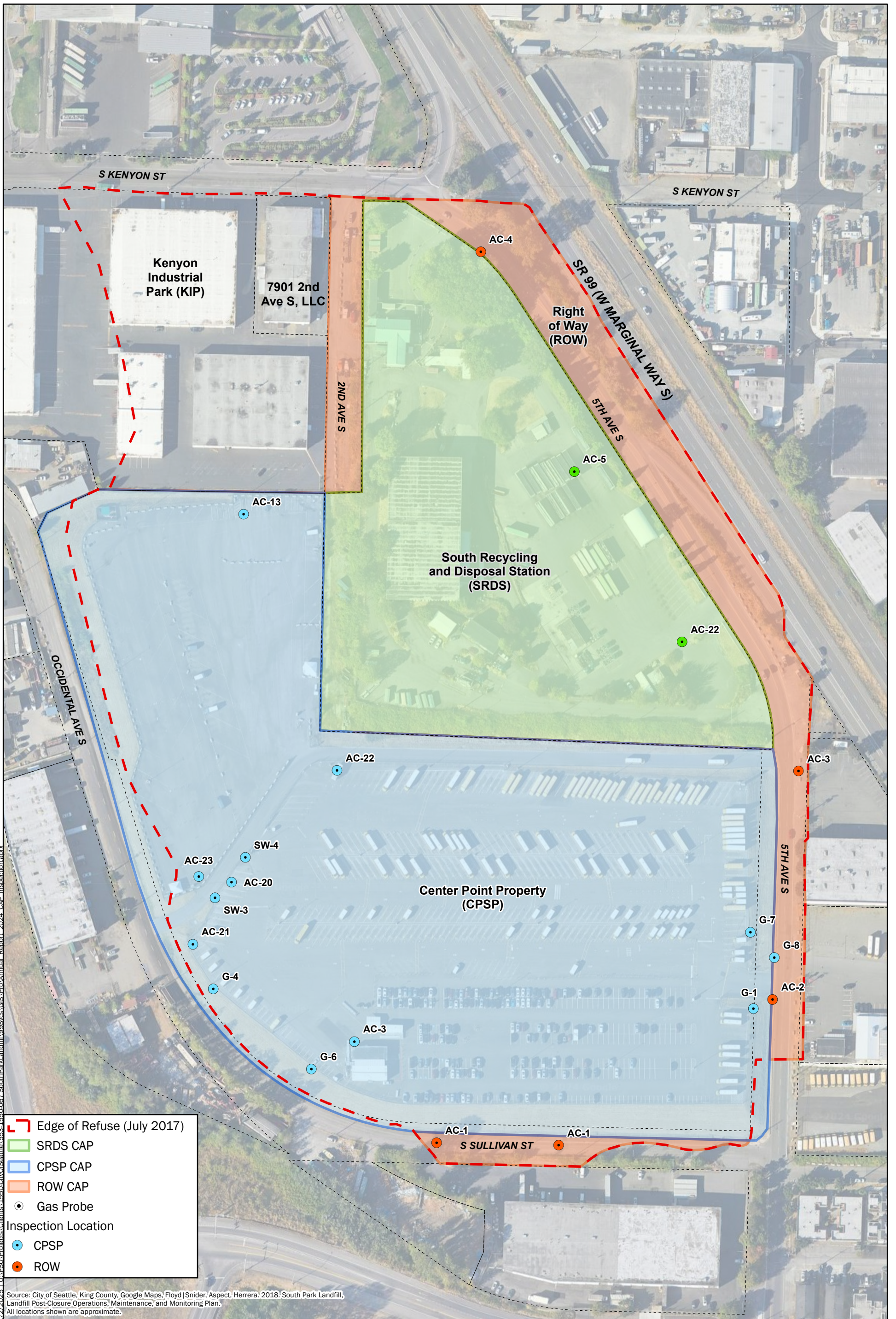
Figure 1 Landfill Cap Inspection- October 2024 Site Plan With Locations for Repair South Park Landfill Seattle, WA
