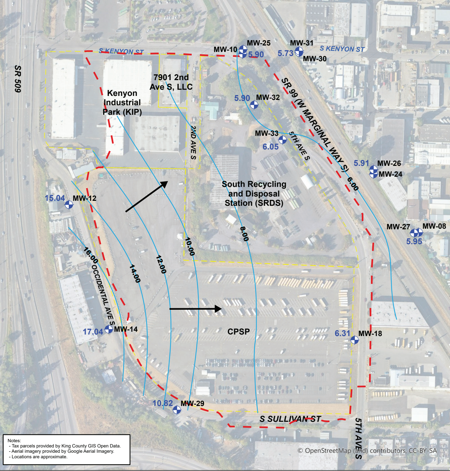
Figure 9 Potentiometric Surface Map November 4, 2024 South Park Landfill Seattle, WA
