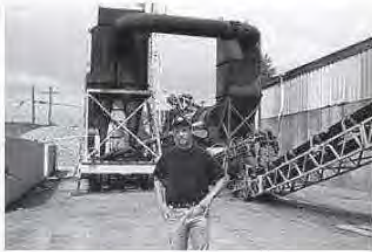
Remedco President Darren Pickering stands in front of his thermal desorption soil treatment plant in Seattle. The plant can treat 50 tons of petroleum-contaminated soil in an hour.
