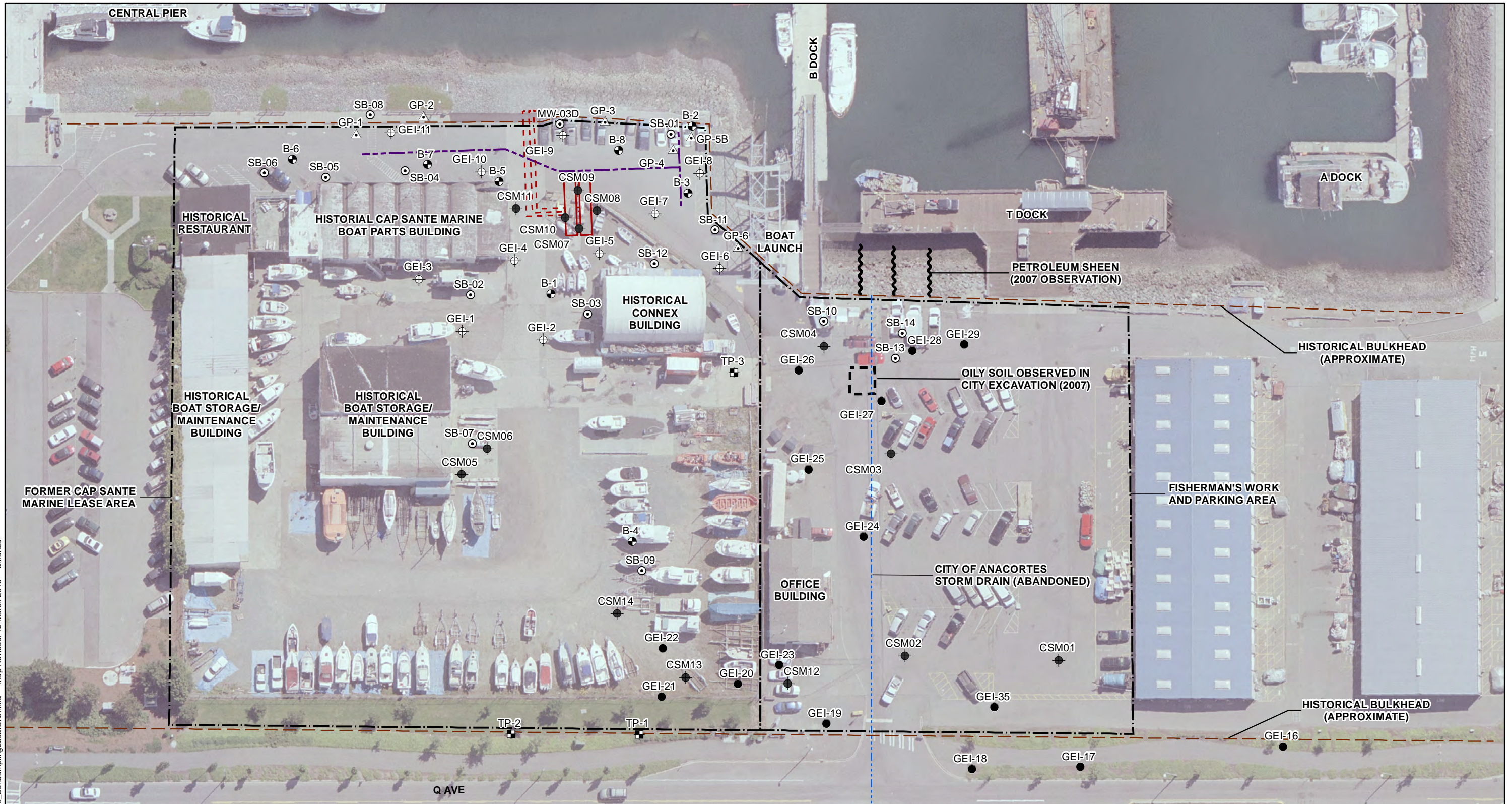
Soil Investigation Sample Locations Cap Sante Marine Site Anacortes, Washington Figure 3
