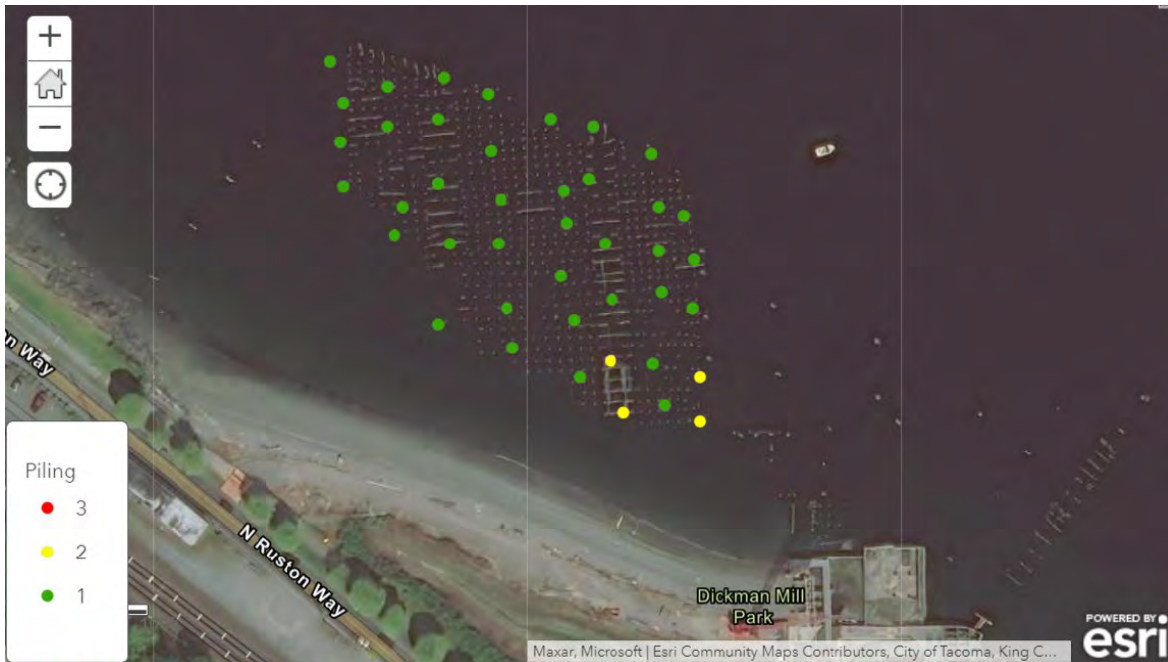
Piling condition rating: 1= not degraded, 2 = moderately degraded, 3 = very degraded
