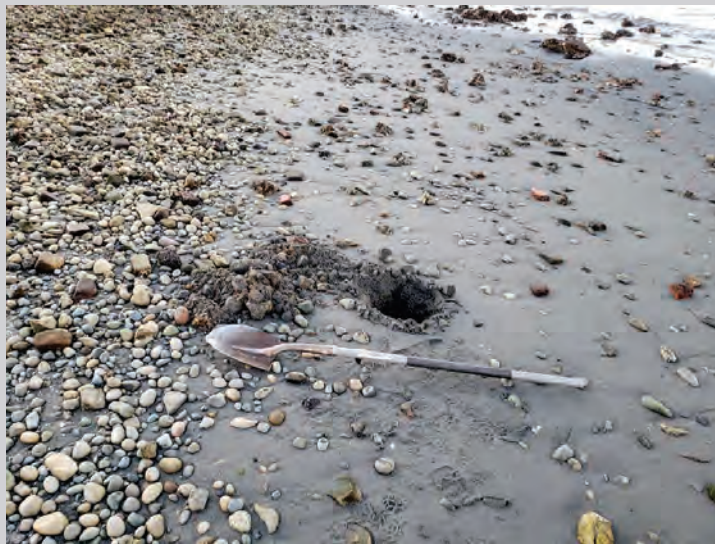
One of two test pits in central cap area with gravel, sand, and shell
