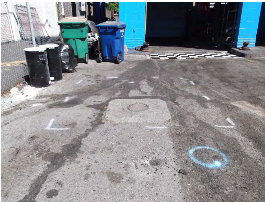
Photograph 6 – View east showing the outline of the apparent UST located west of the northern automotive repair bay. The location of boring KSB-10 is shown by the black patch to the left of the blue circle.
