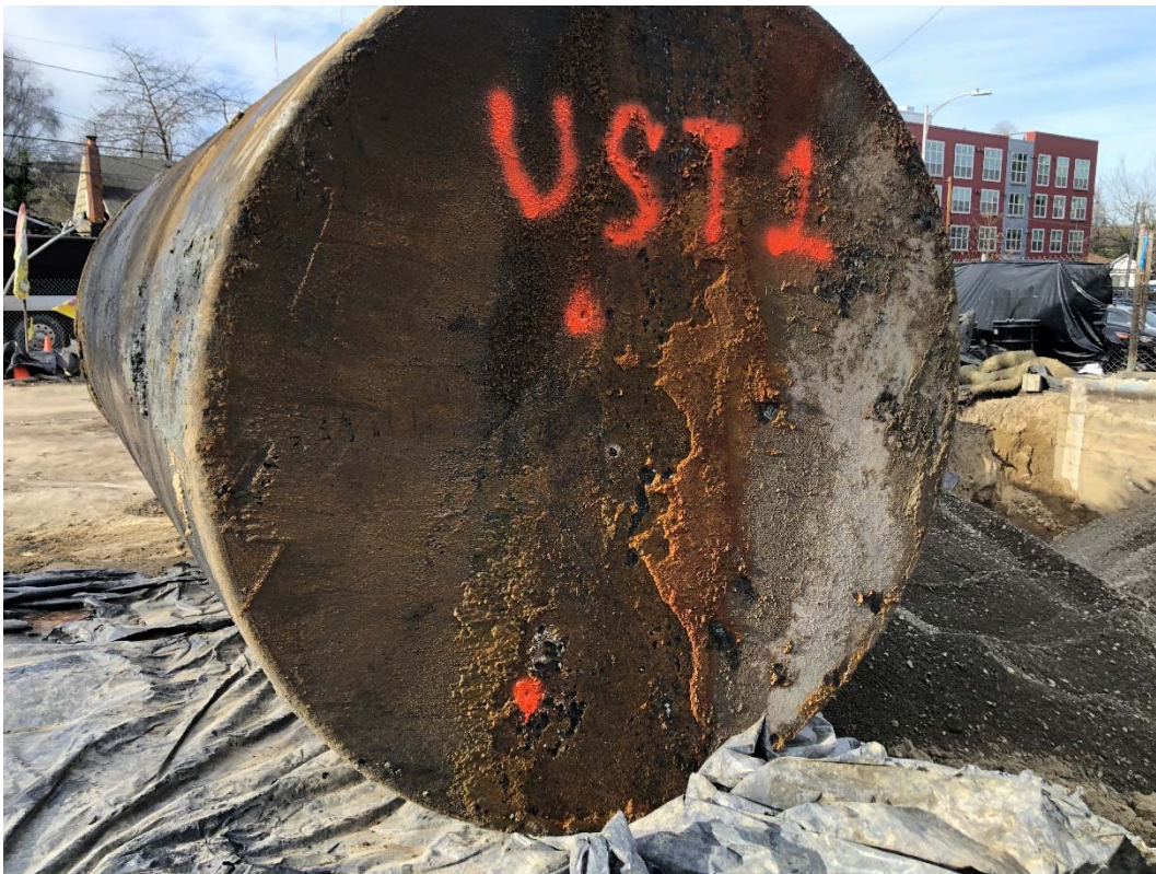
Photograph 12 – View of UST-1 removed from the ground, showing holes in the western wall of the UST painted in orange.
