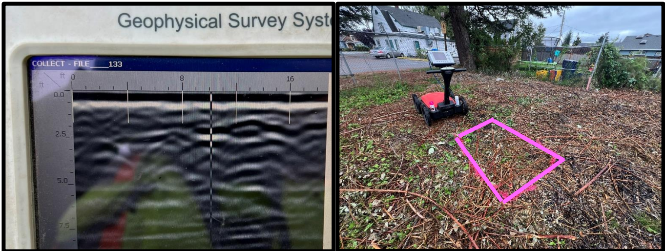
Image 2: GPR cross-section with vertical reference line centered on Anomaly 1 (left). Its observed extent is outlined in pink (right).
