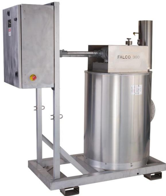
The FALCO 300 electric catalytic oxidizer treats air streams contaminated with volatile organic compounds. The catalyst provides VOC destruction efficiencies up to 99.5%. Operation, including startup, is fully automatic. Control system accurately regulates input loading and temperatures. The controls adjust a FALCO Vapor Control Valve (VCV) to maintain safe maximum input concentrations. Automatic shutdown results if temperatures exceed limits.
