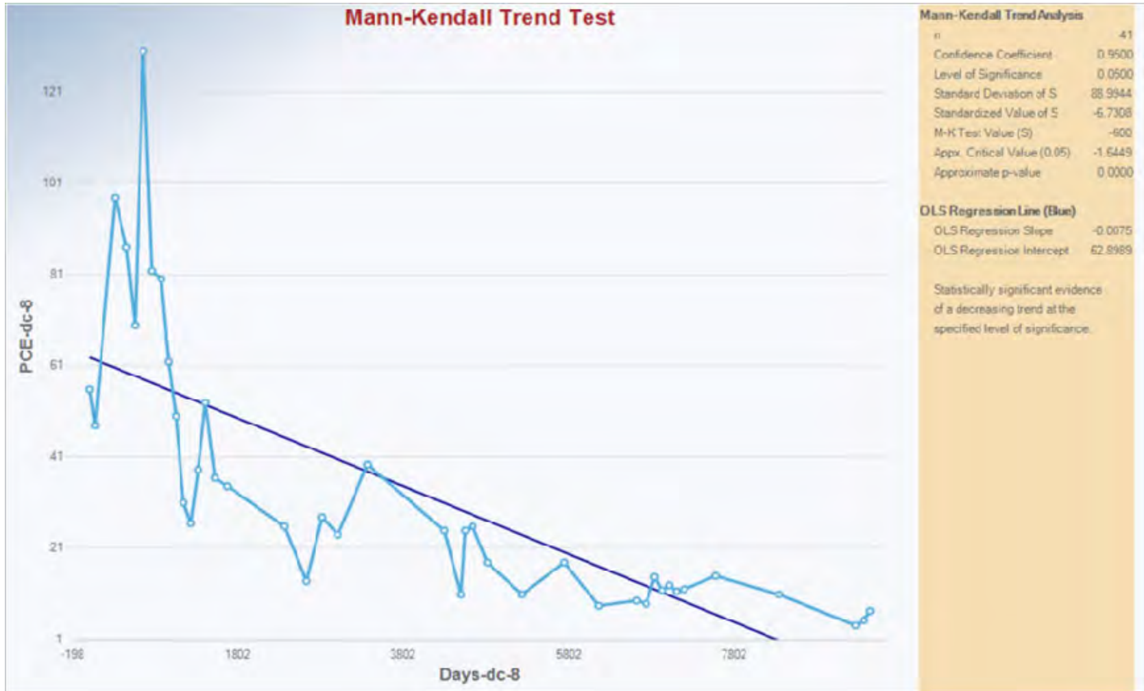
Chart 4 DC-8 Mann-Kendall Trend Test for PCE Manhattan Village Shopping Center and Harris Properties Normandy Park, Washington Farallon PN: 578-002
