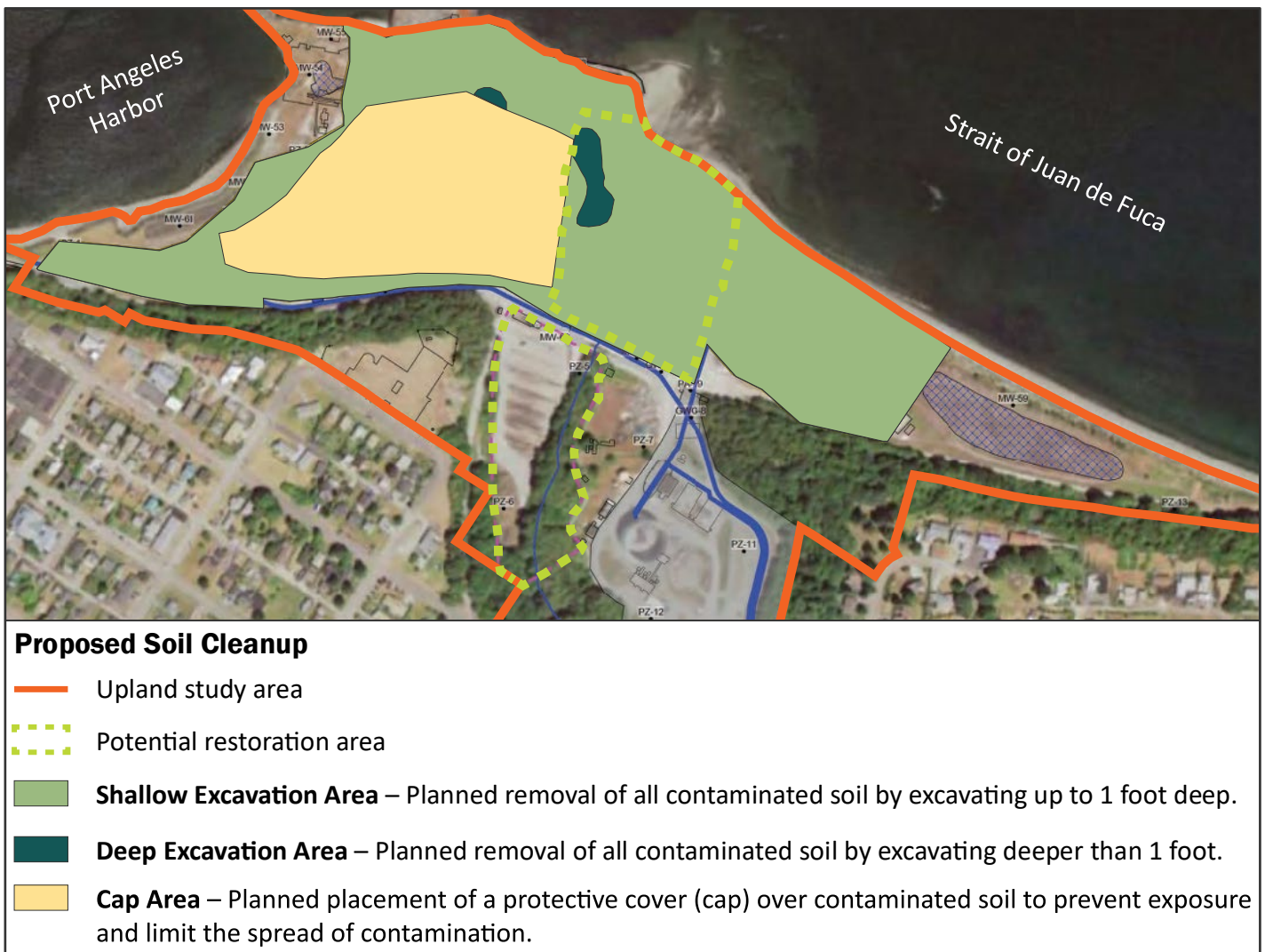
Figure 5: A map of proposed soil cleanup activities. Please note that these are approximate locations.
