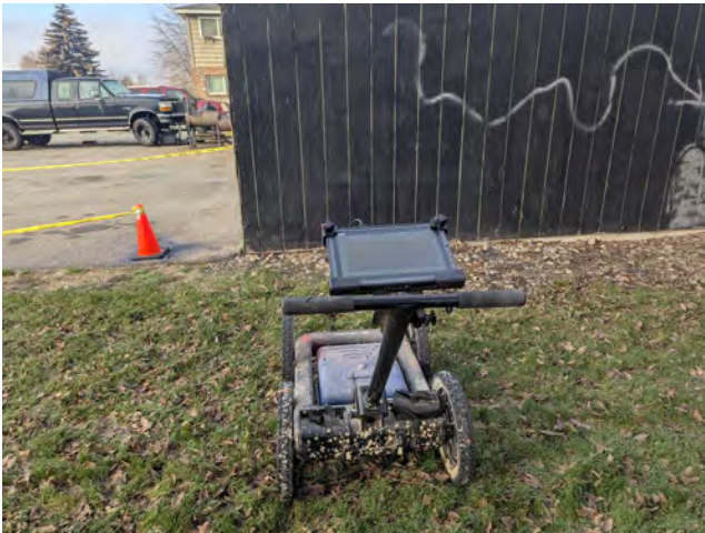
Private utility survey performed via ground-penetrating radar (GPR) throughout Site prior to sampling.
