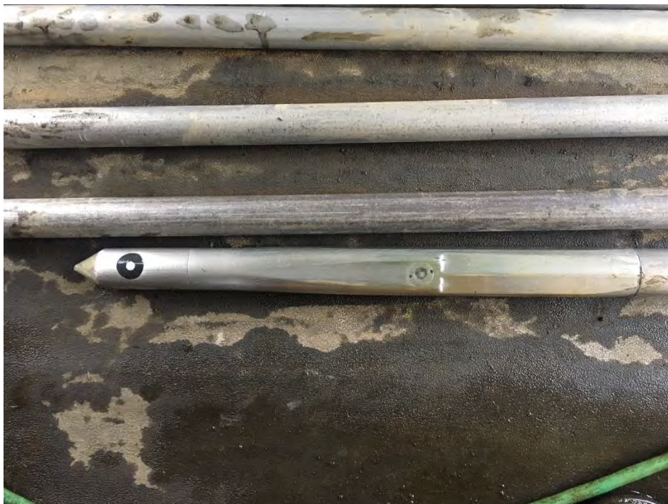
Photograph 2. OIP and HPT probe with rods.
