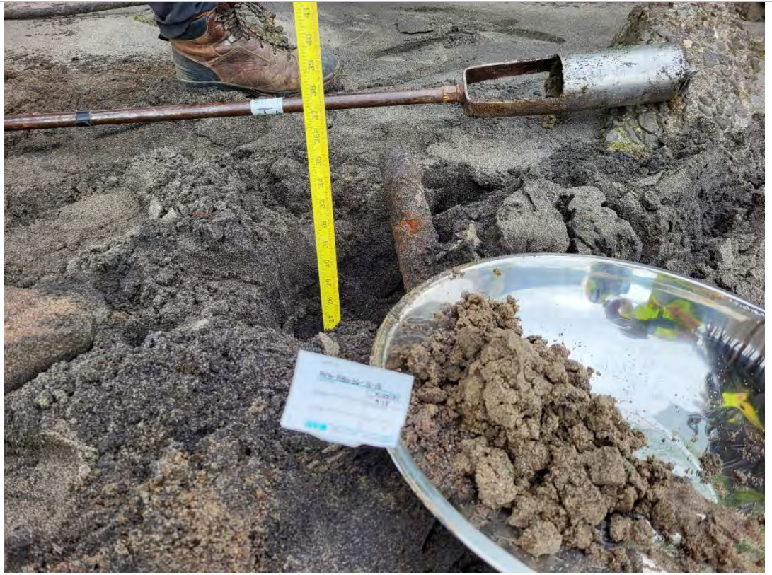
Photo 25 – Sample location and hand augered soil at PNK- RBG35. Metallic debris present.
